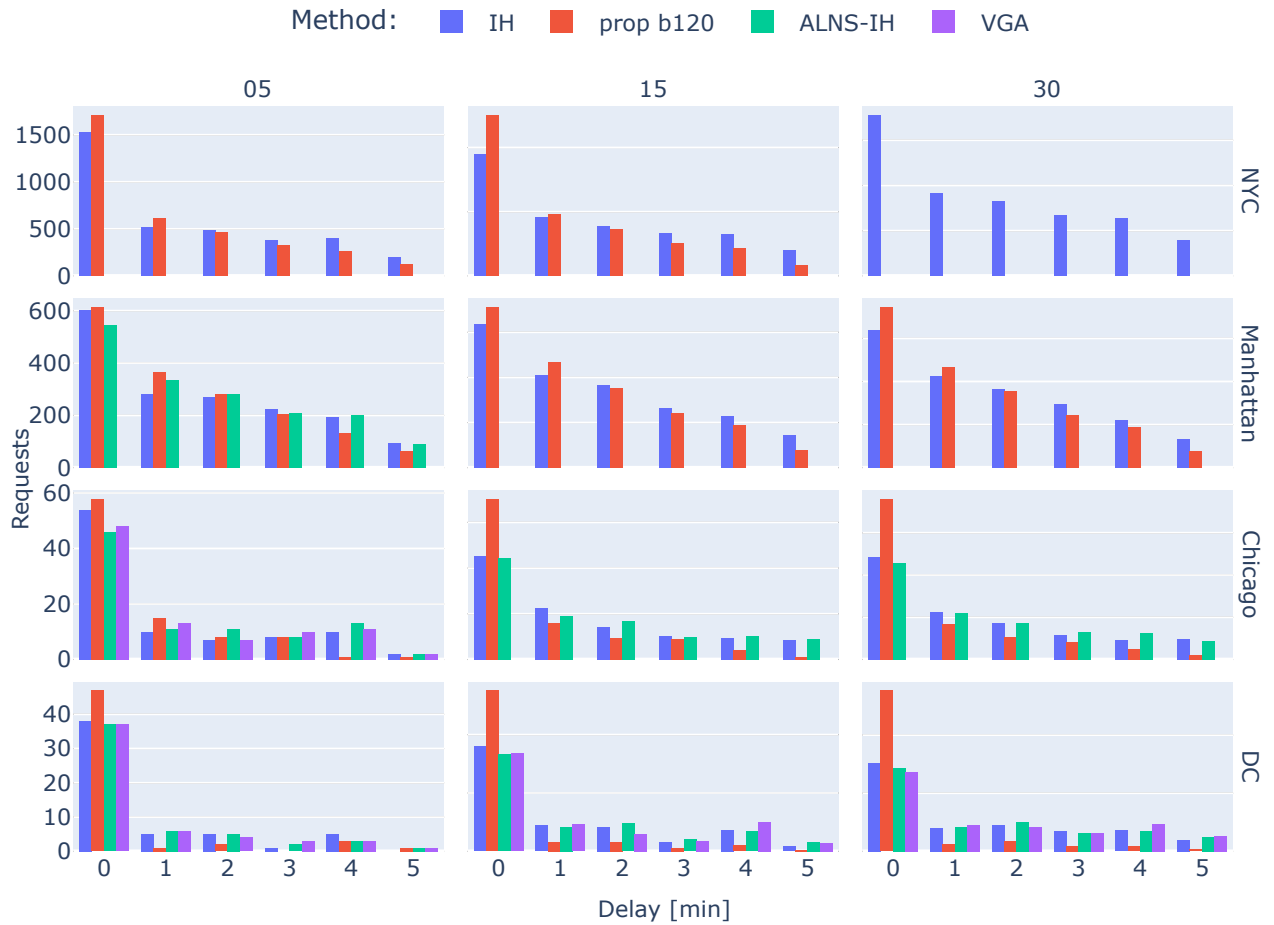
Figure 5.7: Delay histograms for all city-experiment length combinations. The prop b120 method is the proposed method with a batch length of 120 s.
