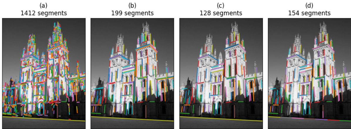
Figure 4.4: Stages of post-processing of detected line segments: (a) output of the LSD, (b) filtering by length, (c) filtering by location, (d) split of long lines.
