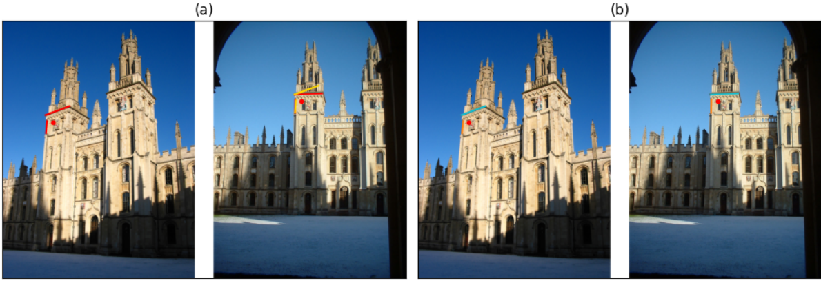
Figure 4.6: An example of a segments matching. In (a), the detected (red) and projected (yellow) lines are depicted. In (b), the established matching is visualised.
