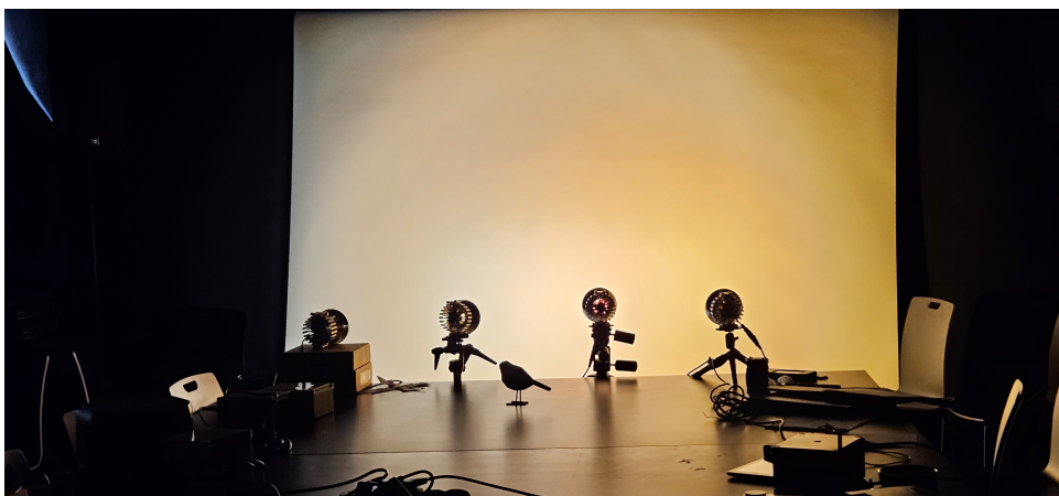
Figure 5.5: Light sources connected to the control system pointed to a canvas - setup for measuring light spectrum of mixed LEDs. Photo courtesy of the NAKI group.
