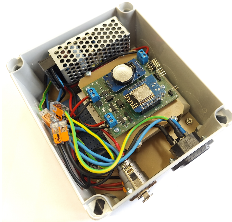
Figure 5.1: Physical realization of the proposed DALI gateway. The module with ESP 8266 microcontroller and DALI bus circuitry can be seen on top. Photo courtesy of the NAKI group.
