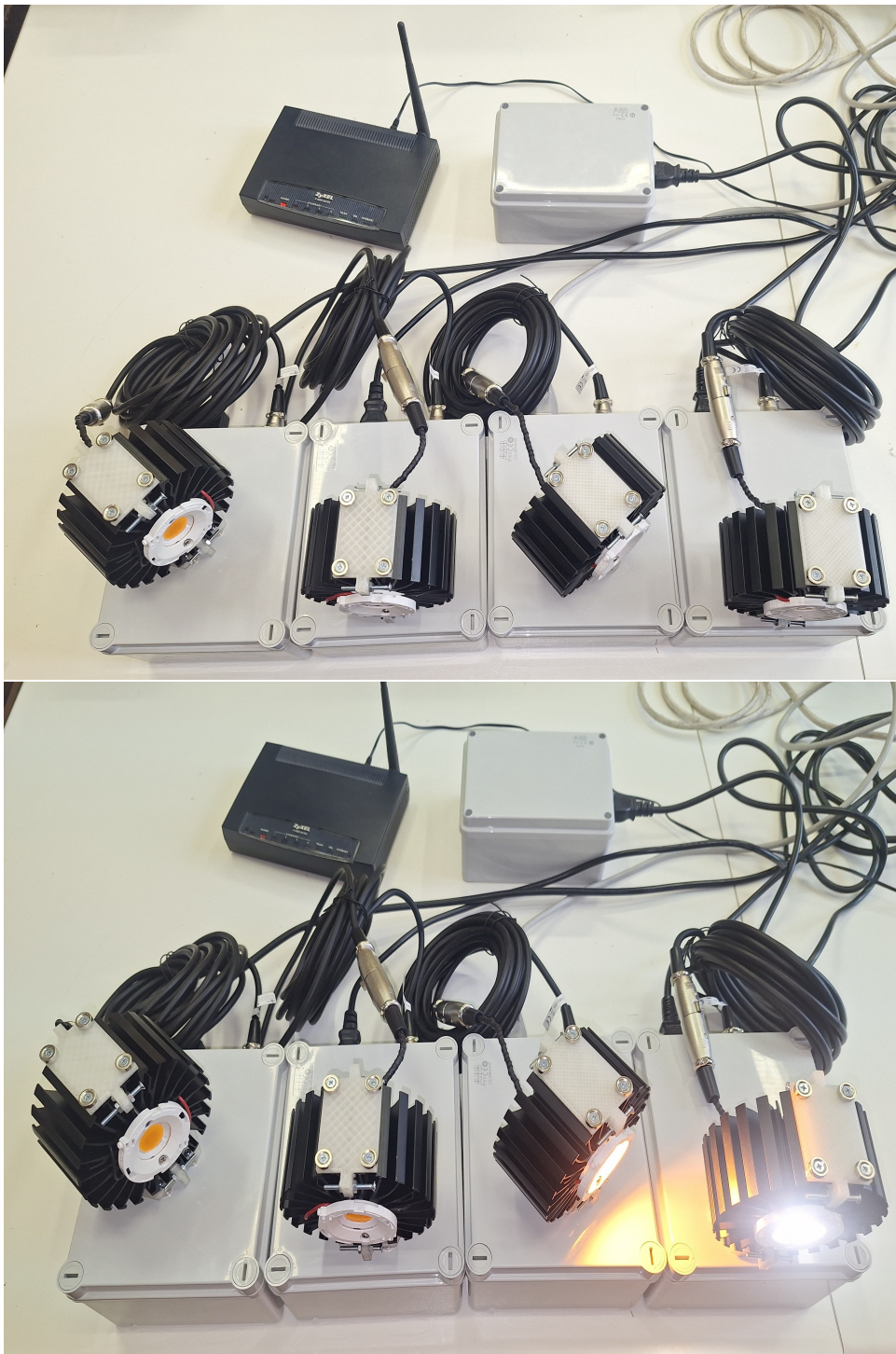
Figure 5.2: Completed setup with four driver boxes a Raspberry Pi box a Wi-Fi router and LEDs. Photo courtesy of the NAKI group.
