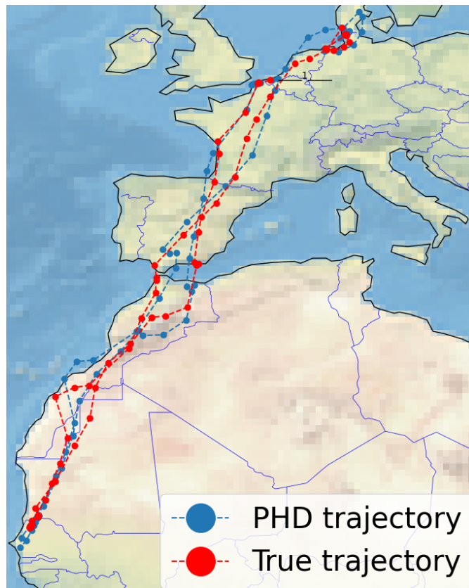
■ Figure 5.4 Comparison of true and PHD trajectory of Ava in clear environment.
