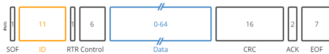
■ Figure 2.2 Structure of CAN2.0 A frame
