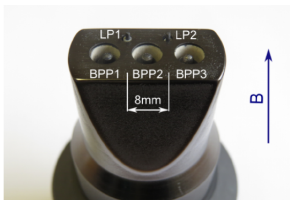
Figure 2.3: The probe head used by the horizontal reciprocating probe. It carries two Langmuir probes (LP) and three ball-pen probes. [21]
