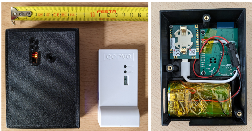
(a) The front of the tag with the holes for the status LEDs (b) The inside of the tag for human
