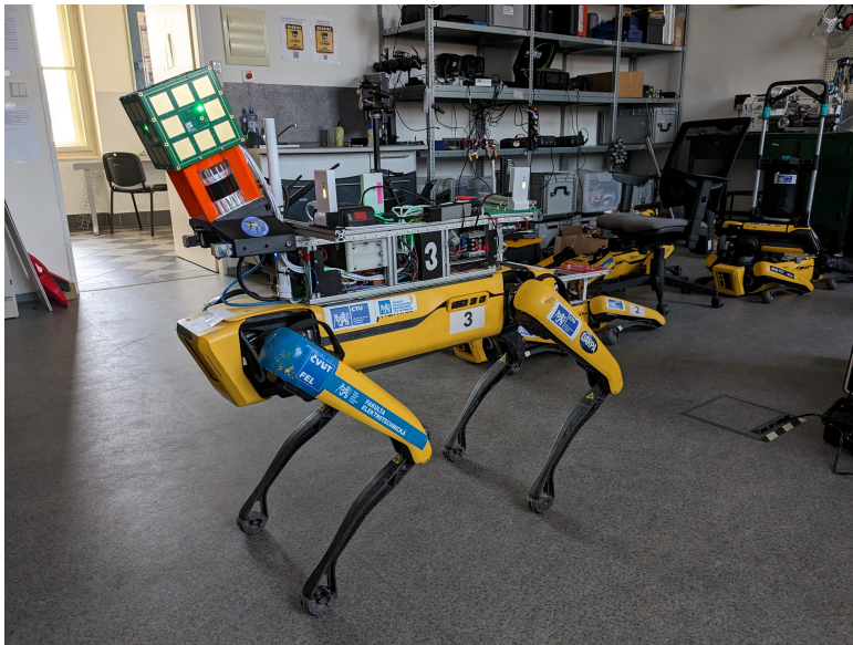
Figure 3.19: The four Bluetooth antenna boards mounted as a single cube on top of Ouster OS-0 LiDAR on Spot robot.
