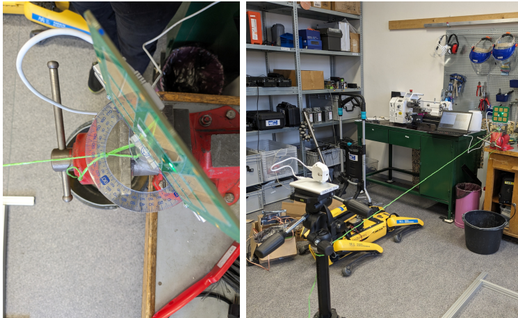
(a) The ANT-B10 antenna (b) The Bluetooth tag placed 2 meters away from the ANT-B10 antenna mount.
