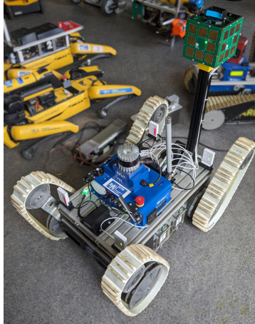
Figure 5.3: The tracked robot with the UWB modules mounted in the corners of the top plate, there is also a cube of AoA antennas mounted on a rod above the body of the robot.
