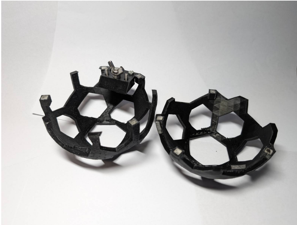
Figure 3.2. Photo of the 3D printed probe fixture. Photo author.
