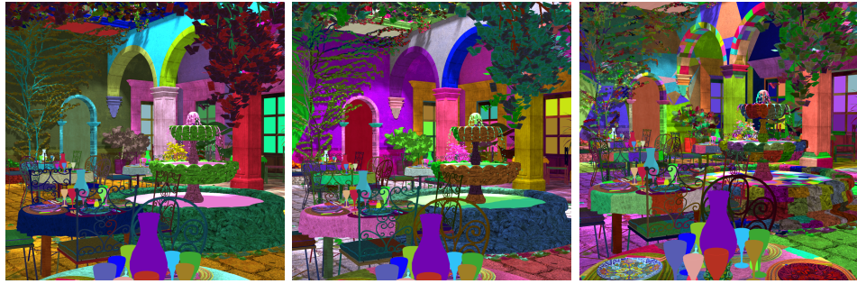
Figure 5.2: Fragmentation of the San Miguel scene is shown in random diffuse color per mesh. Left original scene, center BVH 10^{-4} , right BVH 10^{-1}
