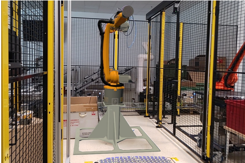
Figure 4.17. Holograms of the robot's and sanding spindle's models in Hololens 2 headset.
