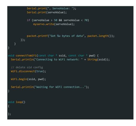
It is necessary to change the Wi-Fi name and password parameters from the beginning to be for the same Wi-Fi as the headset is connected to.
