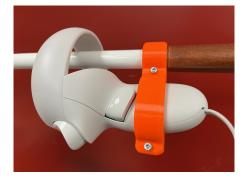
Figure 4.1. The implementation of the real world cane with a controller
