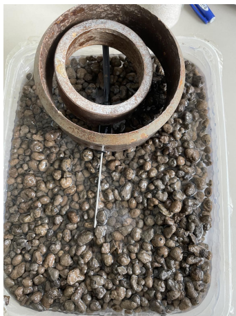
Figure 23: Thin stainless steel probe on the iced substrate
