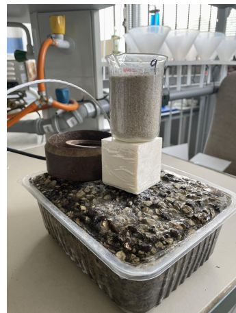
Figure 24: Temperature sensor with aluminium plate and thin stainless steel probe on the iced substrate
