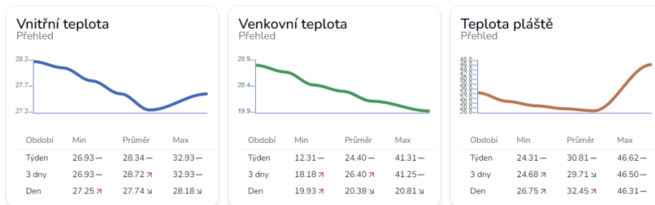
■ Figure 3.11 Partial screenshot of variable overview widgets showing the first 3 variables - chart and minimum, maximum and average statistics over the last week, 3 days and 1 day.
