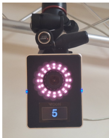
Figure 4.2: Vicon infra-red camera
