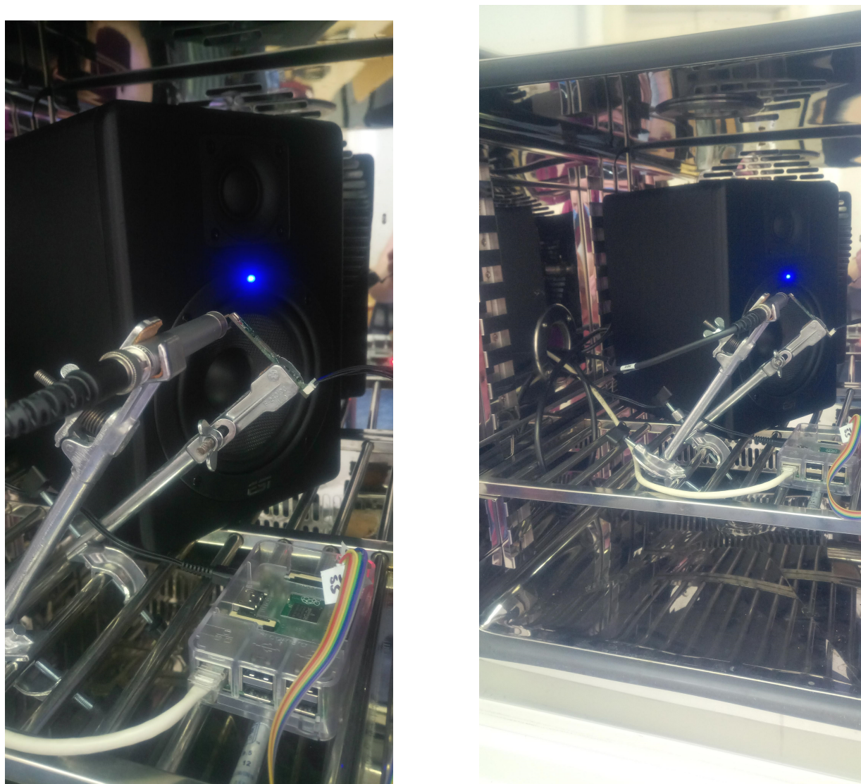
Figure 4.31: The measurement setup: the measured MEMS microphone ICS-43432 placed in the Shjianheng SDJ6005 temperature chamber.
