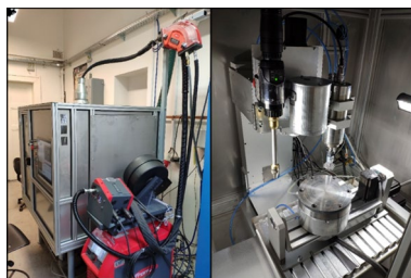
Fig. 11 Experimental WAAM machine setup
