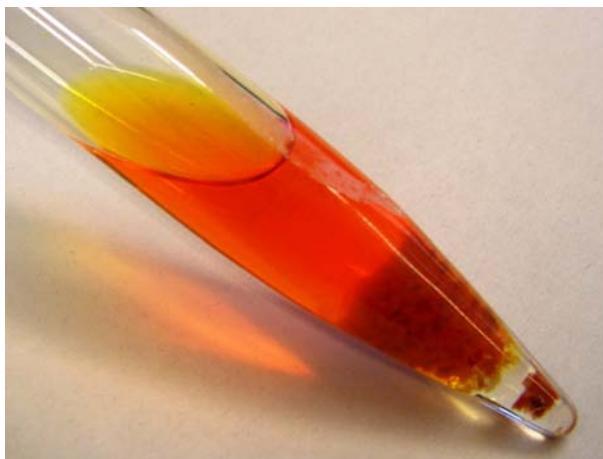
Figure 4 Three-phase (from bottom to top: CS 2 , wood, NaOH) system during the xanthification step.
