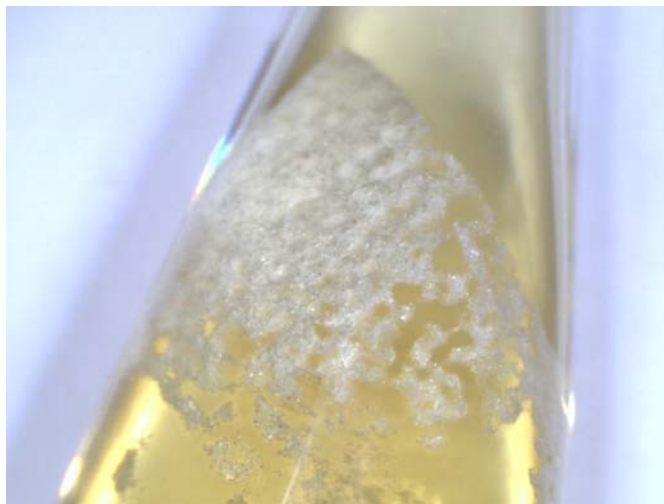
Figure 6 Small piece of C 3 cellulose dissolving in pure [BMIM]Cl at 110 °C
