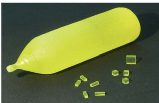
Figure 7. Photo of Gd_3Ga_3Al_2O_{12}:Ce single crystal, diameter 5 cm, length 15 cm. Small optical elements cut from the crystal are shown in the front (courtesy of A. Yoshikawa).
