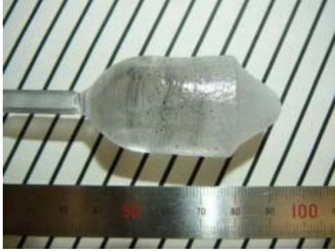
Figure 17. Photo of Ce-doped GPSLa30% single crystal grown by Czochralski technique. (courtesy of A. Yoshikawa)
