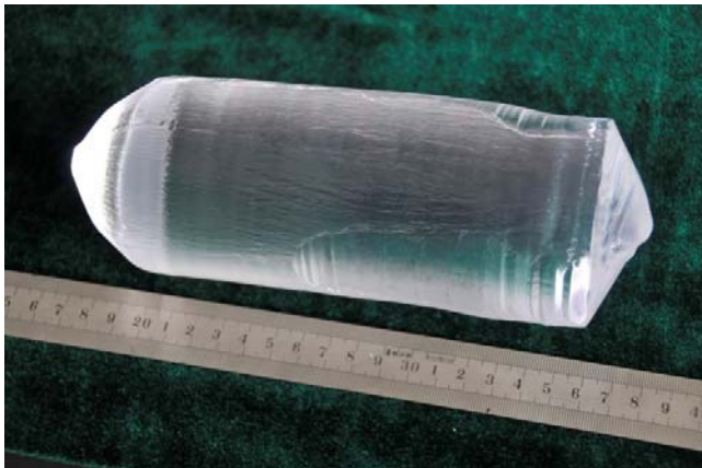
Figure 15. Crystal of LYSO:Ce, diameter 72 mm, length 155 mm grown in Shanghai Institute of Ceramics CAS, China. (courtesy of D. Ding)
