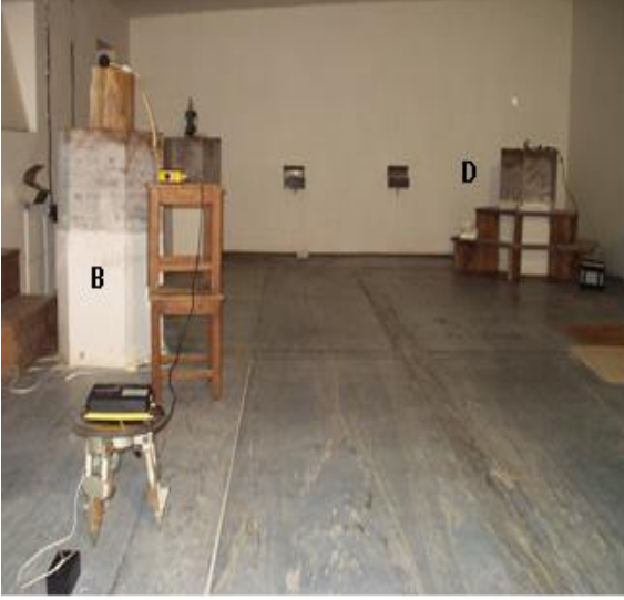
Fig. 2. Actual test setup with the compared magnetometers at the pillars B and D
