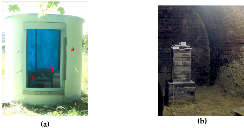
Figure 2. (a) The triaxial sensor head (1) at PLM station is placed in an unheated hut made of PVC (3) and is surrounded by non-magnetic white bricks to increase the thermal mass (2). The hut is painted with special sun-reflecting paint. (b) The sensor at KEL variation station is located 6-m underground.
