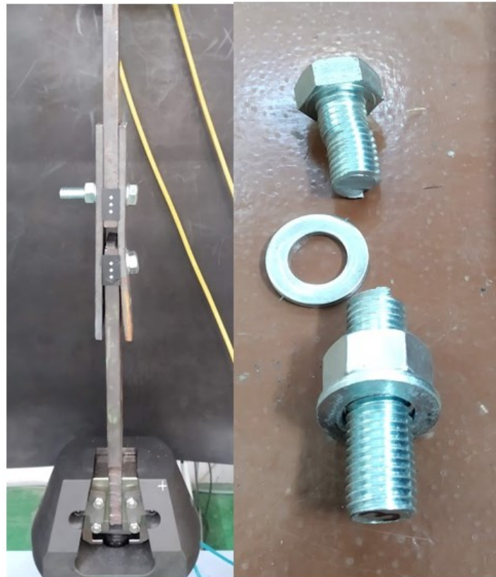
Figure 4.5. Failure modes of tested specimens at 20°C
