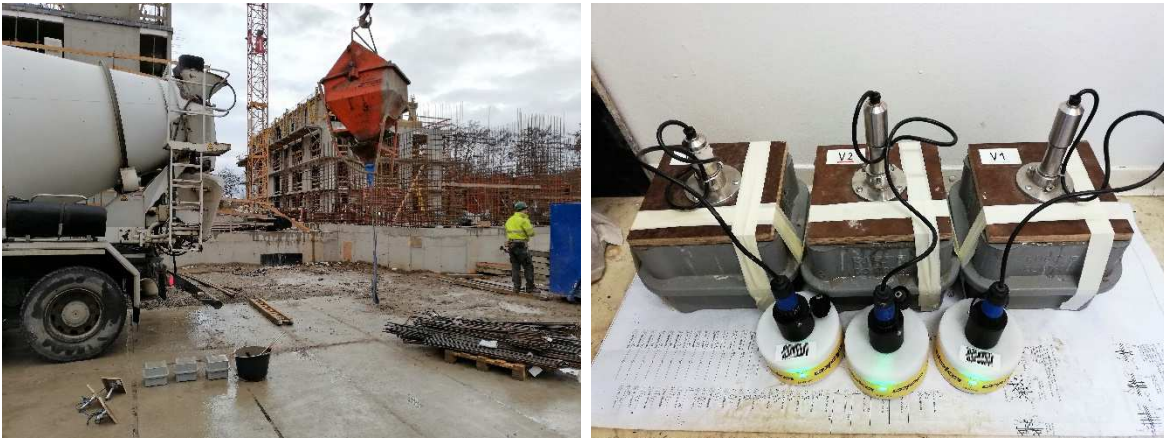
Figure 64 - Prepared samples (left), curing conditions and monitoring (right) [photo: author]
