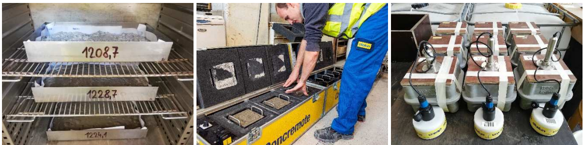
Figure 54 - Determination of w-c ratio, concrete calibration, validation samples [photo: author, R. Syka]
