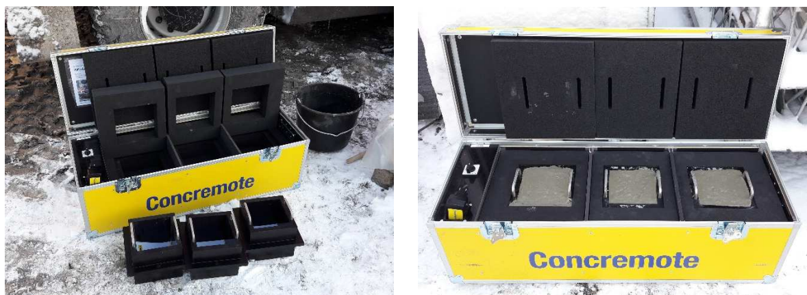
Figure 30 - Example of calibration box, before pouring (left), after pouring (right), [photo: author]
