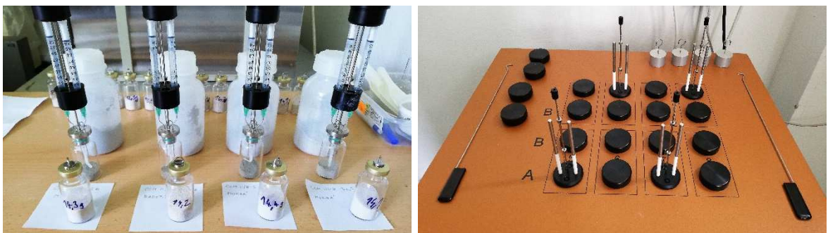
Figure 6 - Samples + reference samples (left), Calorimeter including the samples (right) [photo: author]
