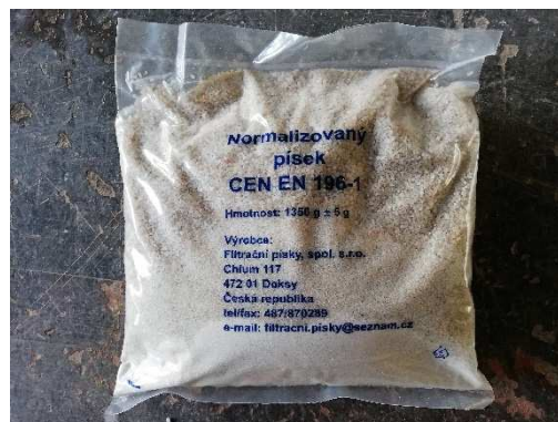
Figure 37 - Plastic bag of standard sand in accordance with EN 196-1 [photo: author]
