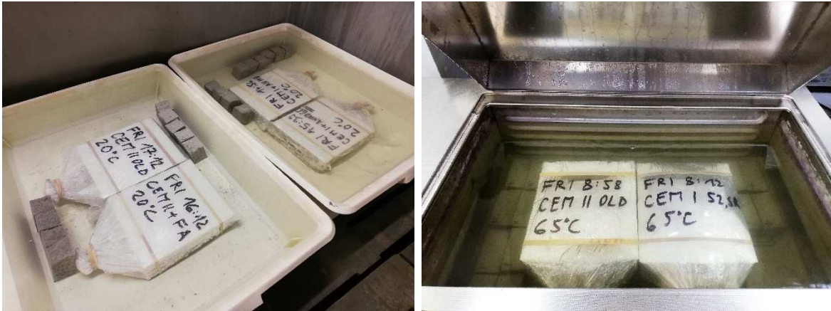
Figure 74 - Determination of C-value - prisms stored at 20°C (left) and 65°C (right), [photo: author]
