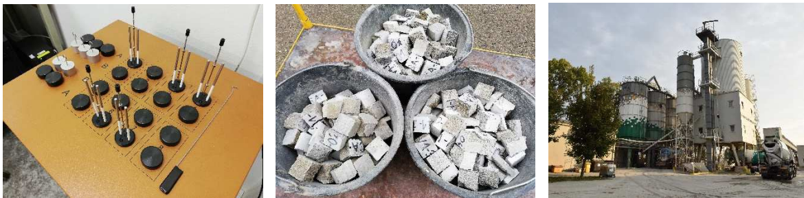
Figure 32 - Isothermal calorimetry test, cement mortar tests, calibrations at concrete plant [photo: author]
