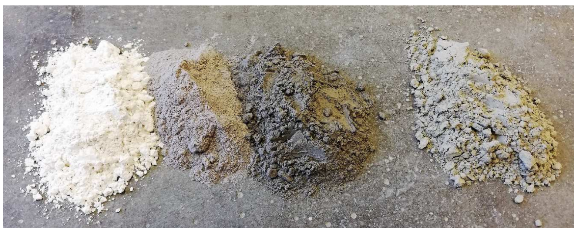
Figure 8 – Cement and additions: limestone, blast furnace slag, fly ash, cement (II/B-S) [photo: author]
