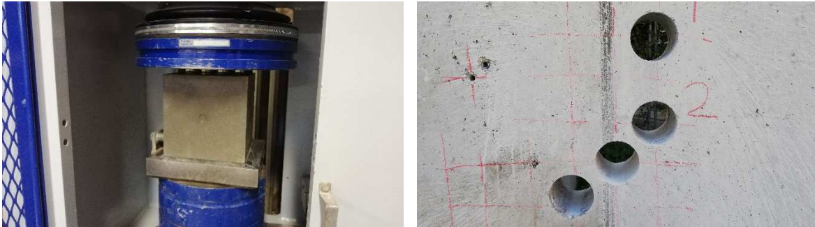
Figure 16 - Compressive strength test (left), structure after cores drilling (right) [photo: author]
