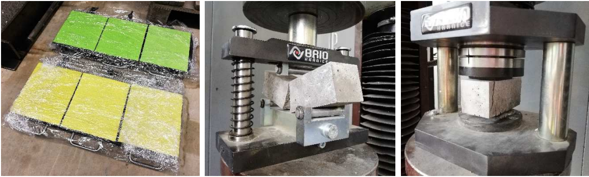
Figure 40 - Curing, flexural strength test, compressive strength test [photo: author]
