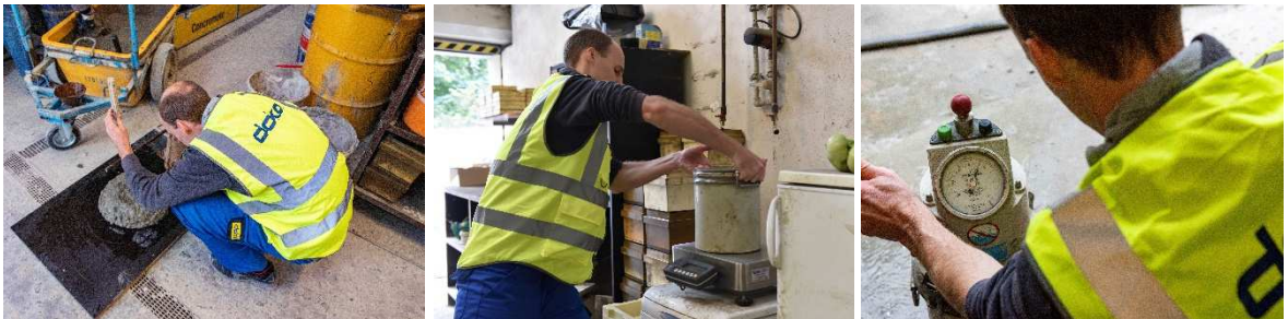
Figure 53 - Slump test, determination of density, air content [photo: R. Syka]
