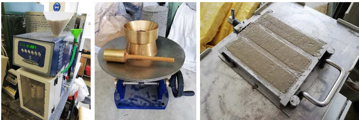
Figure 39 - Mixing of cement mortar, flow cone test, sampling [photo: author]
