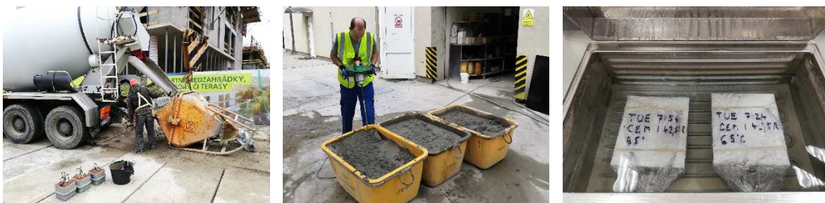
Figure 33 - Validations on the job site, water-cement ratio test, determination of C-value [photo: author]
