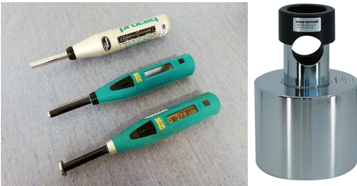
Figure 18 - Schmidt N, SilverSchmidt N, SilverSchmidt L with mushroom plunger [photo: author], testing anvil [51]
