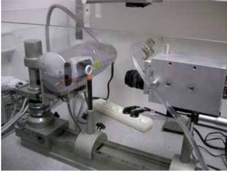
Fig. 2 2D X-ray imaging experiment. X-ray source is on the left.
