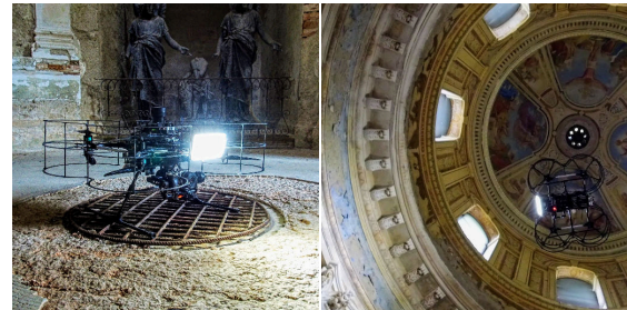
Fig. 2: An application-tailored MAV carrying sensory and mission equipment during documentation of the Klein mausoleum in Sobotín, Czech Republic
