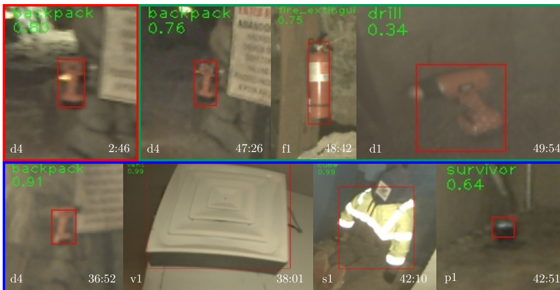
Figure 45. Images of artifacts detected by the UAVs in the Final Event. The color of the rectangle shows which UAV detected the artifact and at what mission time as shown in the bottom right corner.
