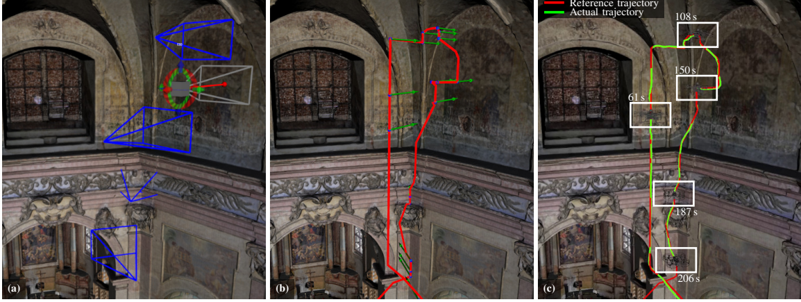
Fig. 3: Pre-deployment phase of the proposed framework — (a) specification of the documentation task by selecting a set of camera viewpoints within the 3D model of the environment, (b) planning trajectory of the robot (in red) which visits all the specified viewpoints (in green), and (c) verification of the mission plan in Gazebo simulator employing identical software that is used during real-world missions.
