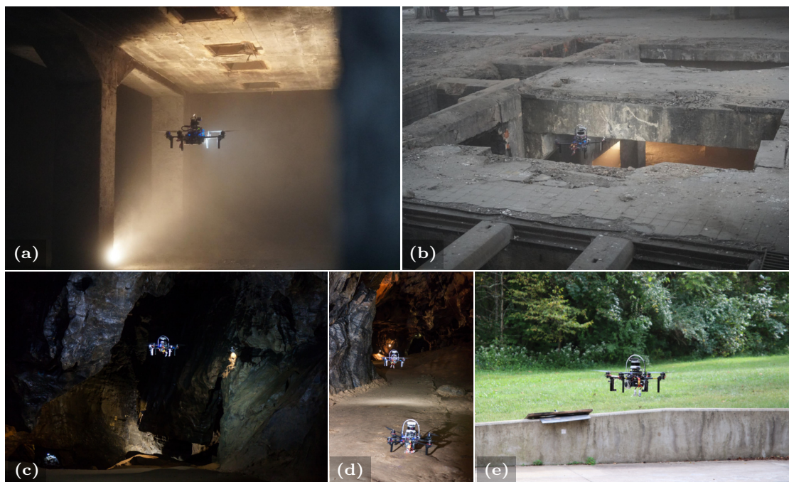
Figure 36. The verification of localization and perception in the following scenarios: data degraded by insufficient lighting and whirling dust (a), traversal of vertical narrow passage (b), performance in humid caves (c), multirobot exploration (d), and scalability with the environment size (e).
