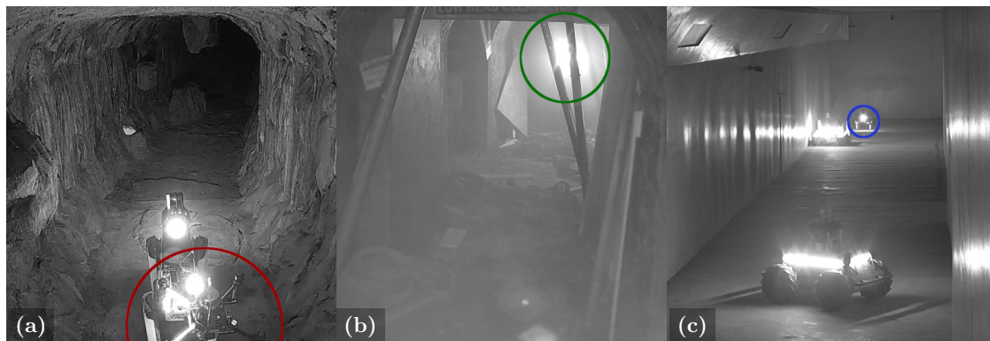
Figure 42. The landing events of all three UAVs. The UAV red (a) collided with the Spot UGV, UAV green (b) hit a metal rod protruding from the wall, and UAV blue (c) landed after its battery was exhausted by hovering while being trapped in a map corrupted by drift in the featureless corridor.
