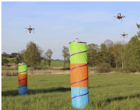
Figure 1. A compact aerial swarm of three UAVs in a controlled outdoor environment filled with artificial obstacles, as viewed by an outside observer. The decentralized approach, described in detail in section 4, applies a set of local rules contributing to safe navigation and self-organization of the swarm structure among obstacles. The UAVs are homogeneous units with solely local sensing.
