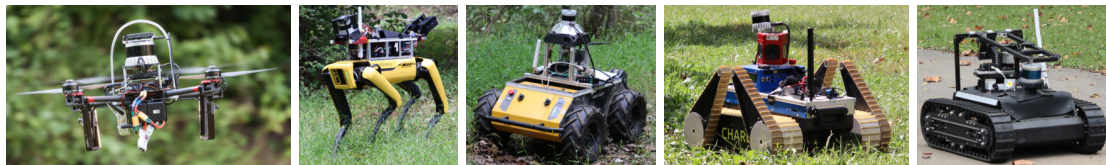
Figure 37. All robotic platforms used in the Prize Round. (From left to right) X500, Spot, Husky, TRADR, Marmotte.
