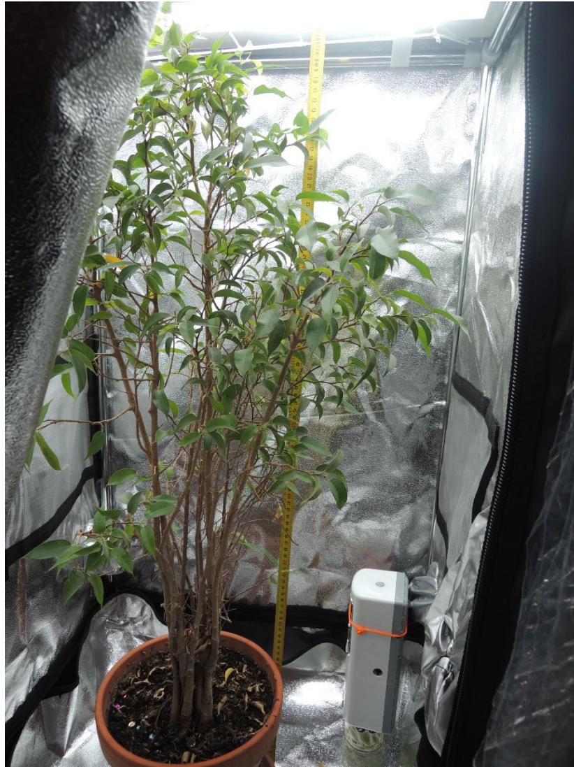
Figure 5-16 Cultivar Ficus Benjamina in a test chamber at an illumination height of 1050 mm
