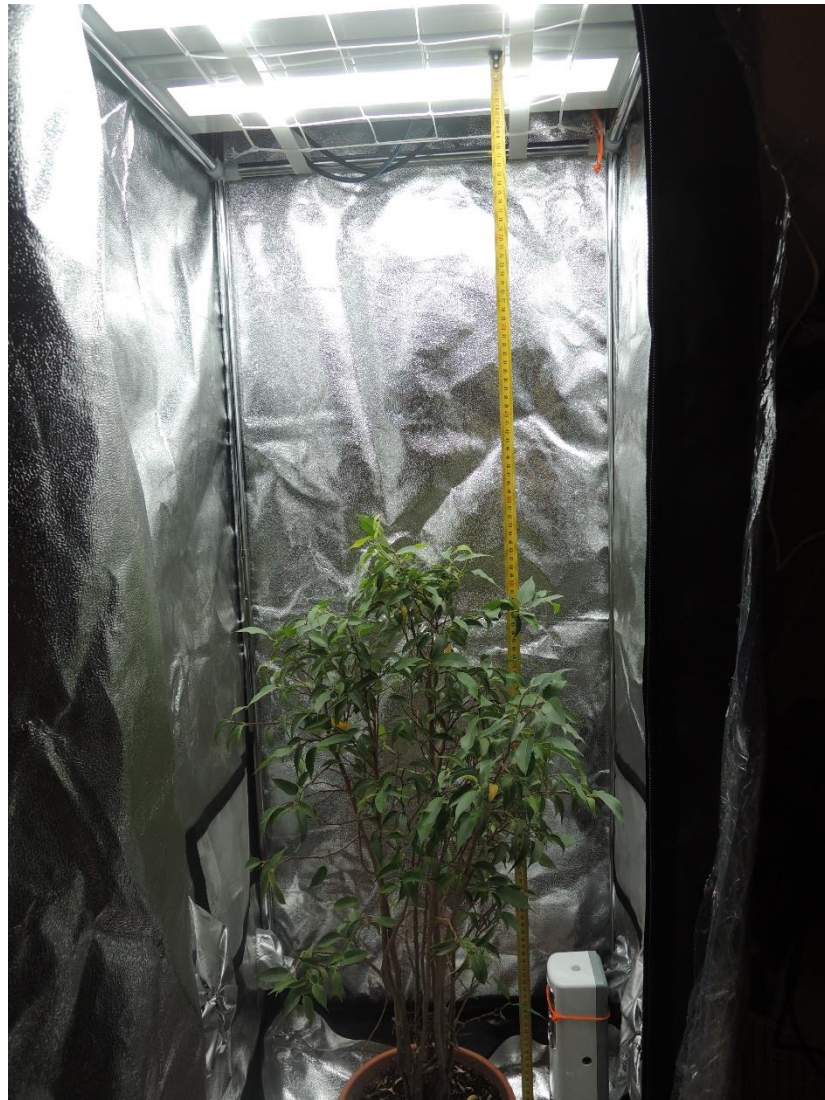
Figure 5-19 Cultivar Ficus Benjamina in a test chamber at an illumination height of 1500 mm
