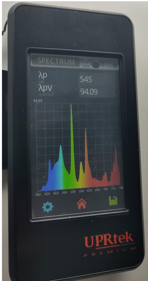
Figure 5-8 Presentation of the spectrum of the artificial light source installed in the test chamber
