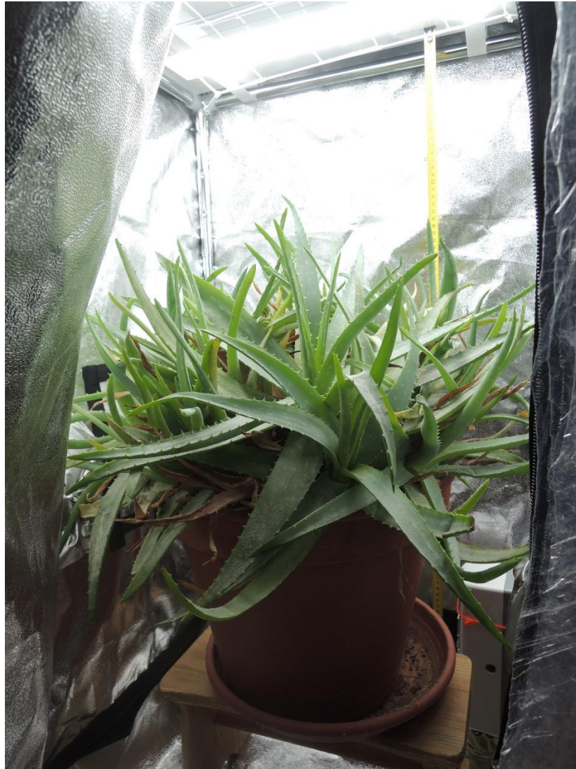
Figure 5-17 Aloe Vera cultivar in a test chamber at a lighting height of 1050 mm
