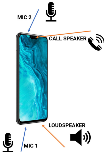
Figure 1 Schematics of the HONOR 9X smartphone audio inputs and outputs.
