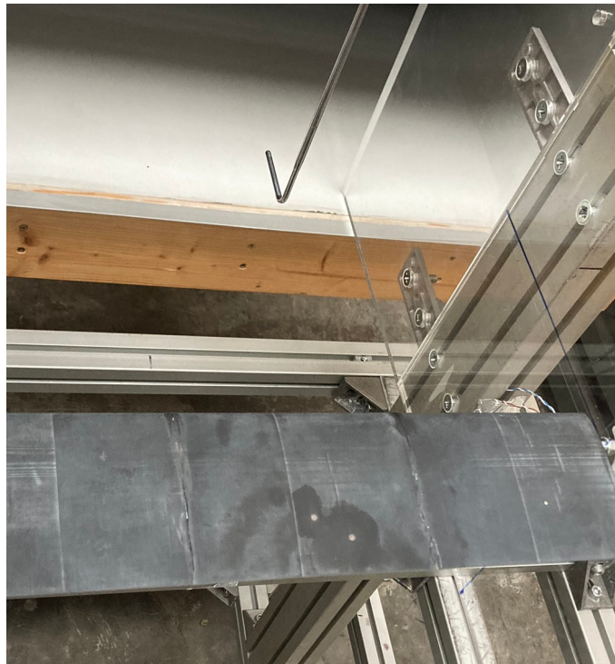
Figure 5.7: The calibration of the airspeed with the Pitot-static probe.
