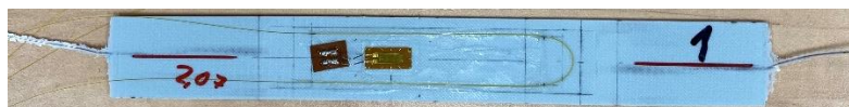
Fig. 70 Specimens with strain gages and optical fibers for distributed sensing installed on the top surface (mold side of the specimen).
