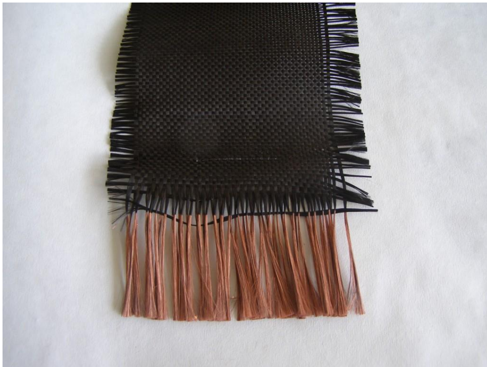
Fig. 118 CF cloth with deposition of copper on several carbon fiber tow
