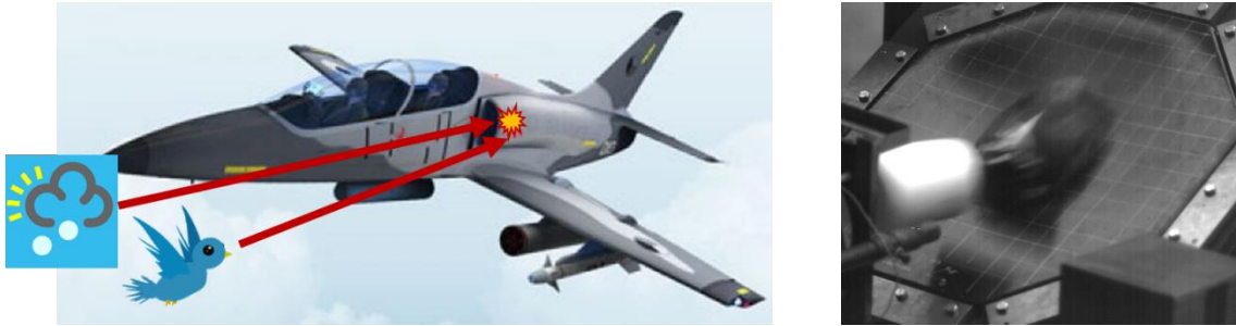
Fig. 45 Possible impact damage scenarios during flight [76] (left); photo from bird strike test of material for aircraft structure [77] (right).
