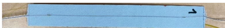
Fig. 71 The specimen with CF sensor integrated between 7 th and 8 th composite layer.
