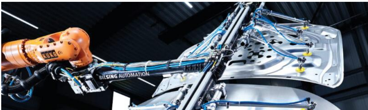
Fig. 104 Filament wound composite profile for the robotic arm [83]
