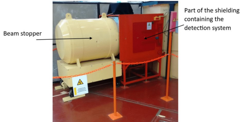
Fig. 2. Shielding of STORNI neutron imaging facility.
