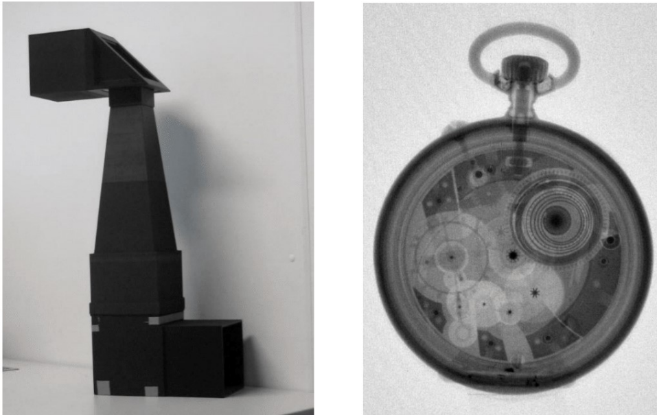
Figure 9. Periscope detector setup (left) for the RA-6 reactor and high resolution radiography (right).
