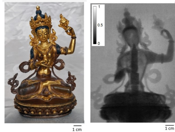
Fig. 2. Photo and neutron radiography of the Bon statue of Sherab Chamma from Tibet.
