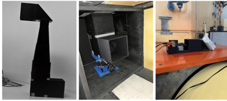
Fig. 6. 3D printed periscope (a) outside the shielding (b) part of the periscope inside the shielding — scintillator box with the first mirror (the scintillator is missing in the photo) (c) part of the periscope outside the shielding — camera box with the second mirror.
