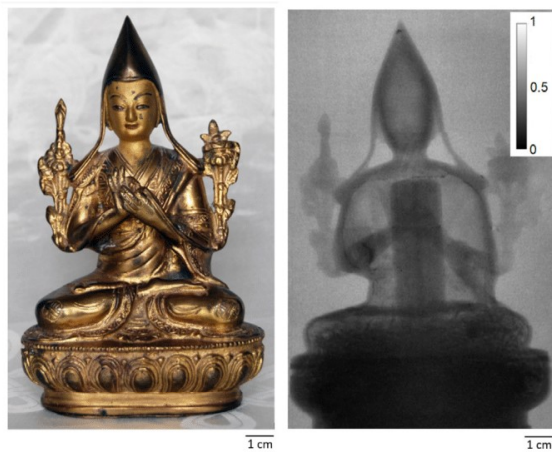
Fig. 1. Photo and neutron radiography of the Buddhist statue of Tsongkhapa from Ladakh in Northern India.
