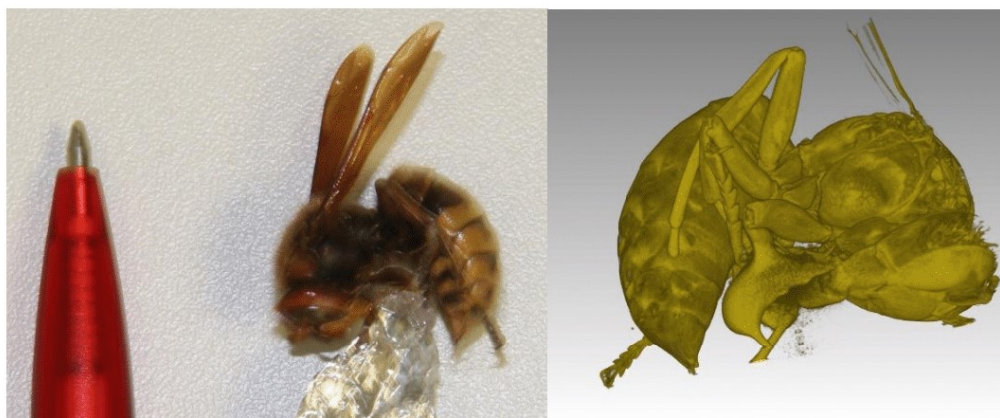
Figure 3. Photo and neutron computed tomography of a dried hornet, with 9 \mu\text{m} effective pixel size. [1]
