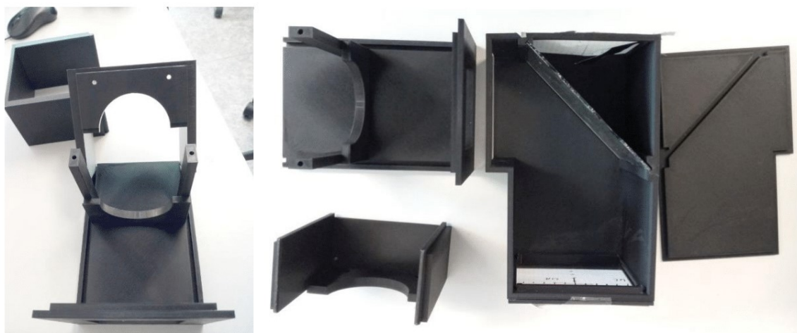
Figure 5. 3D-printed parts of the camera box and the mirror box. The mirror is held by rubber cords pressed into the holding groove.
