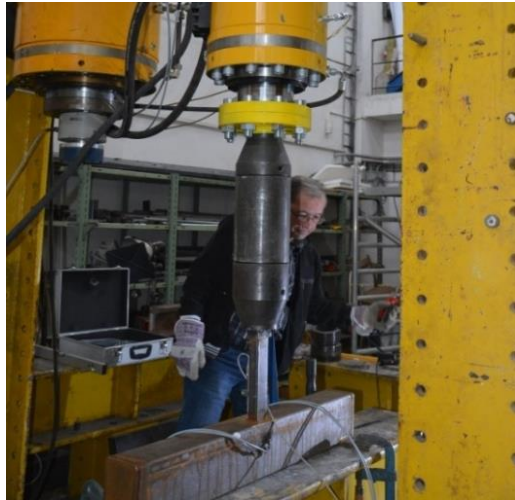
Figure 4.1 Test setup of the T-joint specimens
