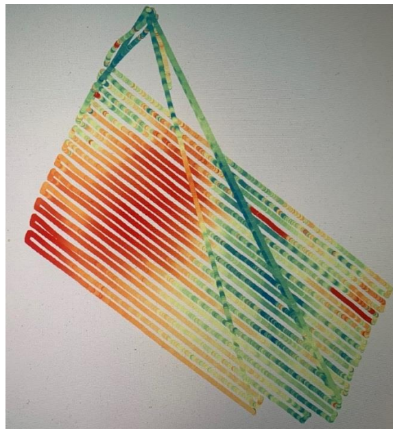
Figure 24. An example of magnetic mapping done with the UAV-MAG (author: Marian Takač)
