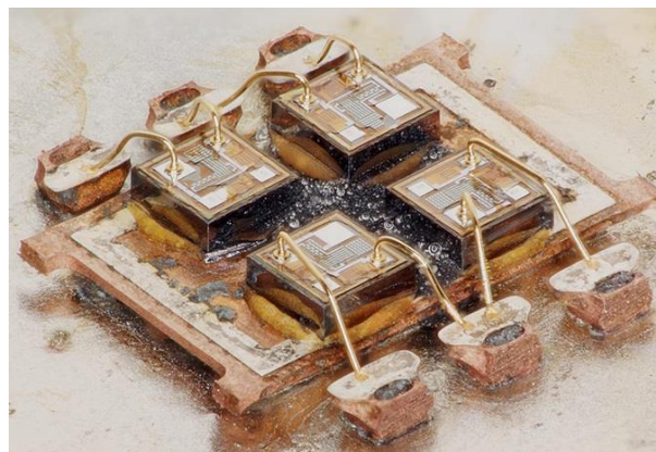
Figure 3. An interesting multi-chip inner structure of a modern TMR sensor, source: Yolo SystemPlus, 2023
