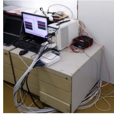
Fig. 12. Photograph of PXIe frame with PC in control room during irradiation.
