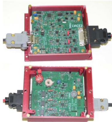
Fig. 6 Fluxgate magnetometer electronics prototype, PC104 format.
