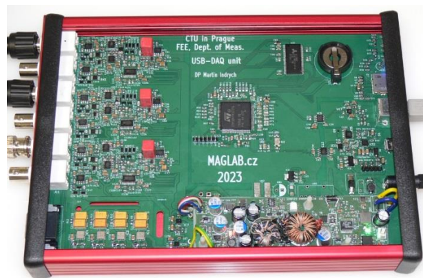
Figure 16. The three-channel DAQ module for analog magnetometer output digitization
