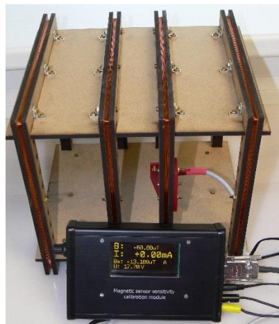
Figure 14 The miniature, single-axis Merritt coil and precise current source for sensitivity calibration of magnetic sensors – used, for example, during noise measurements to quickly estimate sensor sensitivity - developed within the scope of the bachelor thesis Rais 2023 [76]).
