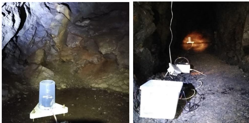
Figure 35. The magnetometer placed at the very end of “Kristýna” stola near Kašperské hory, Czech Republic (the seismologic observatory of the Geophysical institute, Academy of Sciences of the Czech Republic). A 12 V LiFePo battery was used to power up the magnetometer and universal RS232 datalogger to capture the data.
