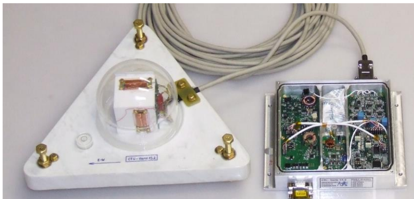
Figure 1. The presented variometer – left: the triaxial race-track fluxgate triplet mounted on MACOR holder on marble base plate, right: the electronics (cover removed).
