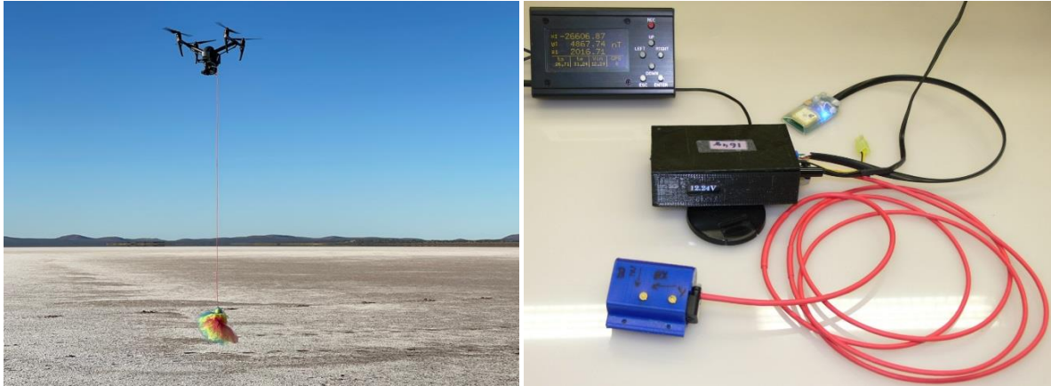
Figure 23. The UAV drone with a 2m-long, flexible boom with the fluxgate magnetometer sensor head. The colored skirt stabilizes the sensor head during flight, improving data quality. The set of the UAV-MAG is shown in the right-hand picture – in the top-left is a ground unit for setting-up the measurements with a control display, in the middle is the magnetometer’s electronics box with the attached GNSS module while the smaller, blue box is the triaxial sensor head. (Left photo by Marian Takač)
