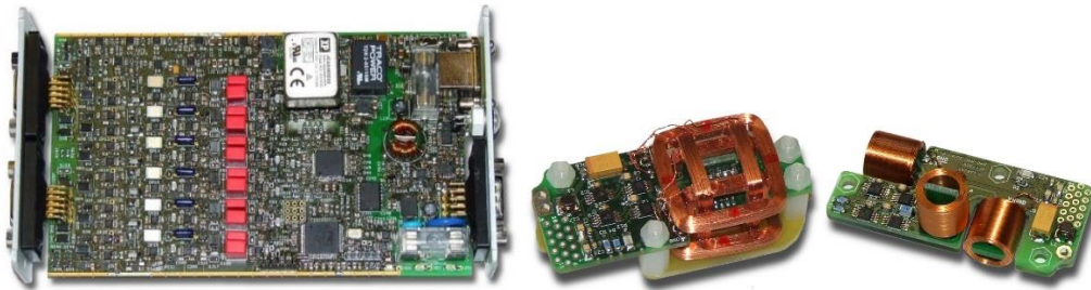
Figure 17. An AMR-based, dual triaxial vector magnetometer with a traditional analog signal processing followed by a high resolution ADC. Right: two sensor heads developed by the author - one with vectorial compensation of the measured field, another with an individual compensation using external coils to provide a more homogeneous compensation field and better coil constant.
