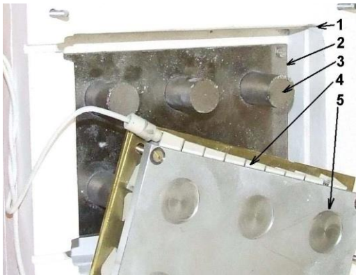
Fig. 2 Photograph of the annealing furnace. "1" is the thermal insulation made of Duratec 750 (bottom, side walls, and top). "2" is the steel plate that fixes the permanent magnets and acts as a yoke in the bottom part of the furnace. "3": Six SmCo permanent magnets generate the magnetic field. "4": Heating is provided by ceramic elements with resistive wire. "5": A hard-chromed CuCr alloy plate equalizes the temperature and fixes the annealed ring cores in the desired center position.
