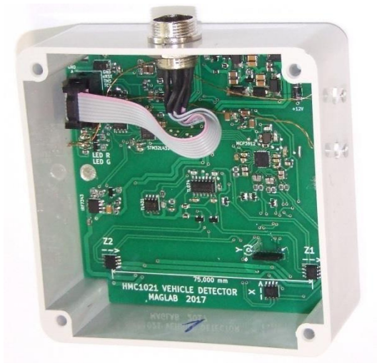
Figure 19. The AMR sensor-based module for car detection experiments, developed under the TACR (Technology Agency of the Czech Republic) project "Advanced Sensors". The module with four single axis AMR sensors was able to measure a magnetic field vector and its gradient in one axis. The author cooperated on its development and testing.
