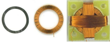
Fig. 6 Construction of the dual-axis sensor is simple: magnetic core (left) is fixed in a fiberglass laminate support, and the excitation winding is made (center). The core assembly is then placed into another FR4 laminate support, and the two pick-up (compensation) coils are wound.
