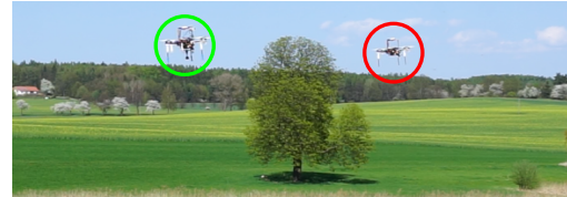
Fig. 11: View of directed leader-follower experiment, the leader (red) is retreating from the follower (green).
