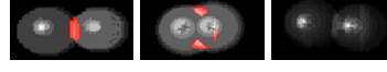
Fig. 4: Erroneous peaks (red) in Hough Transform for pitch (left) and yaw (center), are suppressed by element-wise multiplication.
