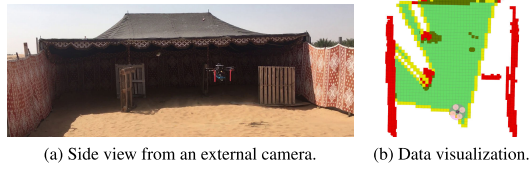
FIGURE 16. Experimental verification of the indoor motion planning and exploration techniques in the desert near Abu Dhabi, United Arab Emirates before MBZIRC 2020. In the image on the right, the red blocks denote obstacles, the green blocks show the already scanned space, and the yellow blocks denote frontiers for exploration. A video from this experiment is on YouTube 12 .
