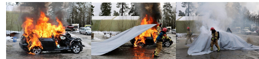
Fig. 2: Fire blanket used to extinguish a burning automobile. The footage was used as motivation for designing the firefighting maneuver presented in this paper. This task can now be accomplished autonomously by an upscaled version of the proposed system.
