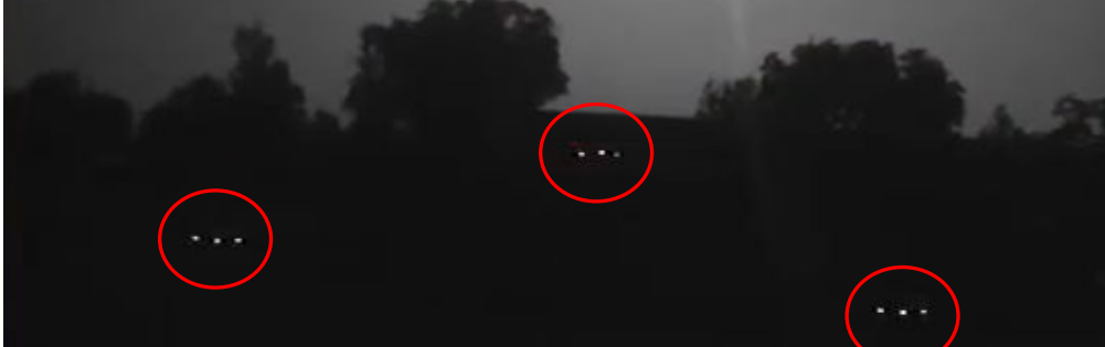
Figure 3: An example of the unprocessed view from the UV-sensitive camera as a part of UVDAR in a member of an aerial swarm. Note the extreme contrast of the LED markers in comparison to the background. A combination of the specific blinking frequency of the LED markers and the high contrast makes them simple to extract from background for processing.
