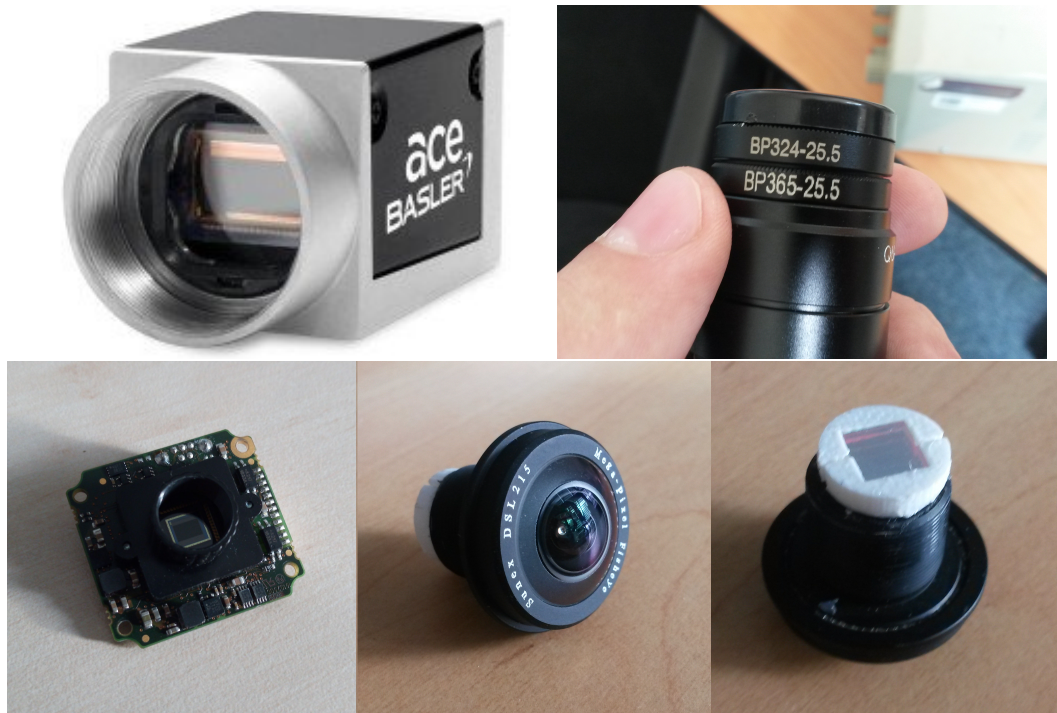
Figure 2.1: Camera and lens equipped with two different ultraviolet filters used in our early tests of ultraviolet vision are shown in the top row. This configuration proved the concept, but was deemed unsuitable for deployment onboard UAV due to size, costs, and incompatibility with fisheye lenses. The bottom row shows the hardware components of our most commonly used and current UVDAR sensor implementation.
