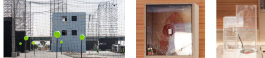
FIGURE 11. Photos of the MBZIRC 2020 Fire Challenge area. The photo on the left shows the tall structure simulating a building, the photo in the middle shows front view of the fire analogues (this unit was turned on) and the photo on the right shows side view of the fire analogues (this unit was turned off).
