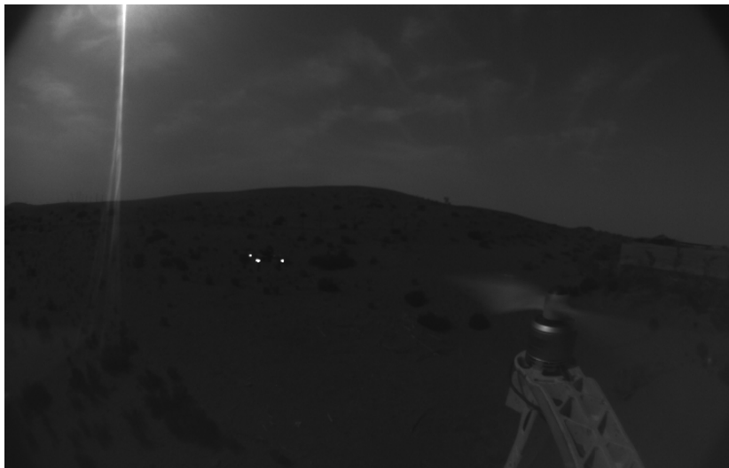
Figure 2.2: View from a UV camera used in the UVDAR system. The three bright dots are the active markers attached to a neighboring UAV. This view is captured in a desert environment at noon, showing the high level of robustness to exterior illumination.
