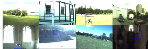
Fig. 1: Examples of annotated footage from the proposed dataset from a disparity of environments. The bounding boxes were generated automatically, using our relative localization system UVDAR .
