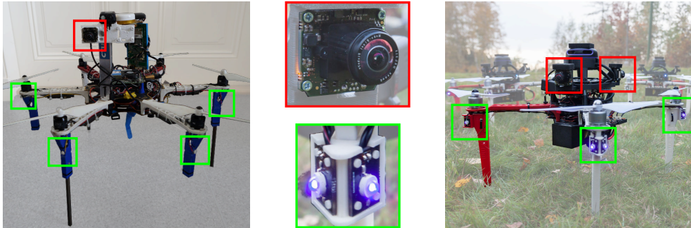
Figure 6: Two distinct multi-rotor (hexa- and quad-rotor) UAV platforms, here equipped with UV-sensitive cameras (red) and with active UV markers (green), comprising the hardware components of the UVDAR system for relative localization of neighboring UAVs. The diagonal dimension (without propellers) of the platforms are 550 mm (left) and 450 mm (right). The hexa-rotor platform was used throughout our experimental verification presented in section 6.
