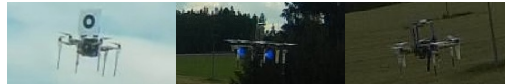
Fig. 2: Experimental platform views, with a passive visual marker (left) [22] and active ultraviolet markers, on and off, (center – left). Without the passive marker, the resemblance to arbitrary MAV is higher, making it more suitable for use in training ML algorithms.
