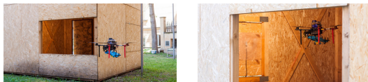
FIGURE 20. Experimental verification of the proposed system on a mock-up of the building set up in the Czech Republic. The image on the left shows the MAV outside the mock-up during its search for an open window. The image on the right displays the MAV while the water is being sprayed on the fire analogue inside the mock-up. A video of this experiment is on YouTube 14 .
