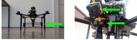
Fig. 3: Front view of the blanket dropping gripper below the body of the UAV (left) and the layout of the thermal cameras (right).
