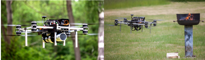
Figure 21. Our working prototype of a firefighting UAV designed for using gas-based extinguishing capsule launcher - an evolution of the system developed for the MBZIRC 2020 competition.
