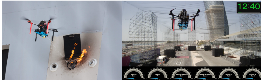
Figure 18. Active extinguishing of a facade fire object in the first trial of the competition.
