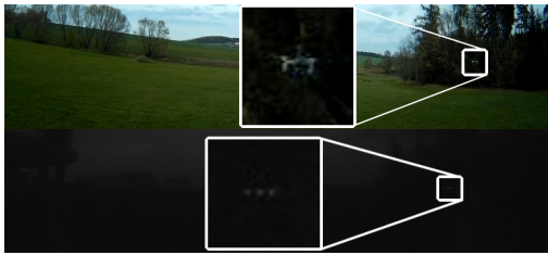
Fig. 3: An extreme case of long range and hard to separate background. In the visible spectrum the UAV is difficult to locate even by the human eye and today's popular CNN methods [7], while in UV the three markers are clearly visible as unique peaks in brightness and can easily be detected by the proposed system.
