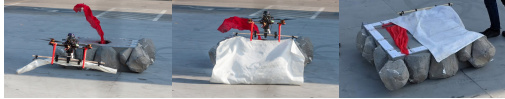
Fig. 9: Our UAV approaching the fire analogue in the placement maneuver. The fire blanket is unrolled when the UAV is 3 m from the target. The second end of the blanket held straight by a wooden rod is released after the target has been covered. The third figure shows the resulting placement - the offset is due to a combination of GNSS drift during the placement maneuver and the blanket sliding off after being placed, due to the air flow from the fire analogue.
