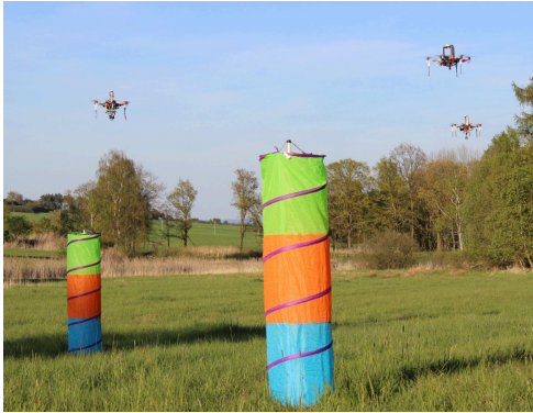
Figure 1: A compact aerial swarm of 3 UAVs in a controlled outdoor environment filled with artificial obstacles, as viewed by an outside observer. The decentralized approach, described in detail in section 4, applies a set of local rules contributing to safe navigation and self-organization of the swarm structure among obstacles. The UAVs are homogeneous units with solely local sensing.
