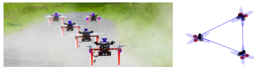
Fig. 1: An example of our fully autonomous Unmanned Aerial Vehicles (UAVs) [1] equipped with the mutual relative localization system UltraViolet Direction And Ranging (UVDAR). The units depicted are based on the MRS F450 platforms. These devices can cooperate using a mutual relative localization and control scheme, such as the one proposed here. The output of the relative localization system is subject to observation noise expressed in terms of covariance of a multivariate Gaussian distribution that is taken into account in the presented method. An illustration of 3D ellipsoids representing the distribution of noise in relative position measurement is shown on the right.
