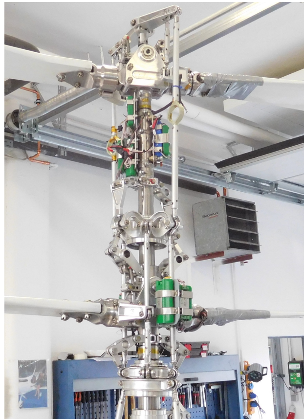
FIGURE 5. Coaxial rotor system of an ultralight helicopter with installed measuring modules.
