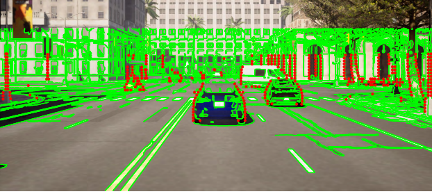
Fig. 8: A frame from the CARLA simulator. LiDAR corners are shown in red, image edges in green.
