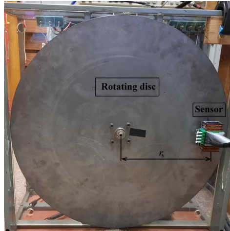
Fig. 11. The eddy current speed sensor and rotating disc as a moving magnetic conductive object
