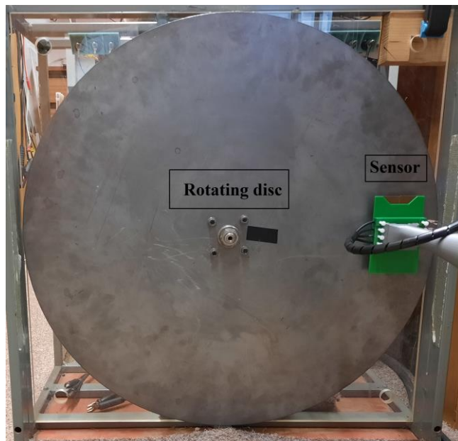
Fig. 10. Eddy current speed sensor with a rotating disk
