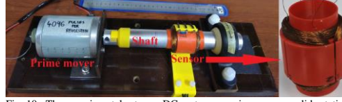
Fig. 10. The experimental set up – DC motor as a prime mover, solid rotating shaft and eddy current speed sensor
