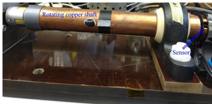
Fig. 11. Experimental elements– with rotating copper shaft and axial airgap eddy current speed sensor
