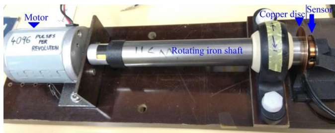
Fig. 15. Experimental elements with DC motor as a prime mover– with iron and copper disc shaft and axial airgap eddy current speed sensor
