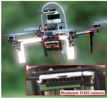
(a) Downward-facing RGBD camera used for landability detection mounted on our UAV platform.
