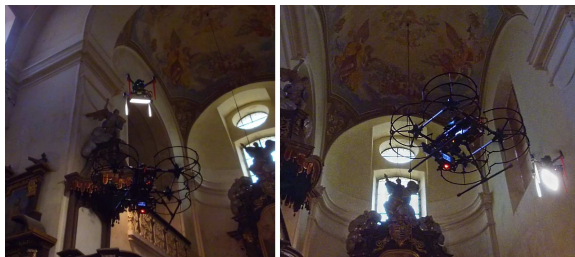
Fig. 2: Deployment of the proposed system for autonomous RTI by a team of UAVs in Church of St. Mary Magdalene in Chlumín. Multimedia material of the experiment is available at http://mrs.felk.cvut.cz/papers/rti2020oral .
