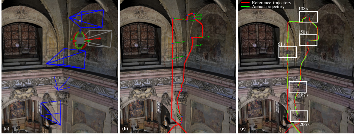
Fig. 3: Pre-deployment phase of the proposed framework — (a) specification of the documentation task by selecting a set of camera viewpoints within the 3D model of the environment, (b) planning trajectory of the robot (in red) which visits all the specified viewpoints (in green), and (c) verification of the mission plan in Gazebo simulator employing identical software that is used during real-world missions.
