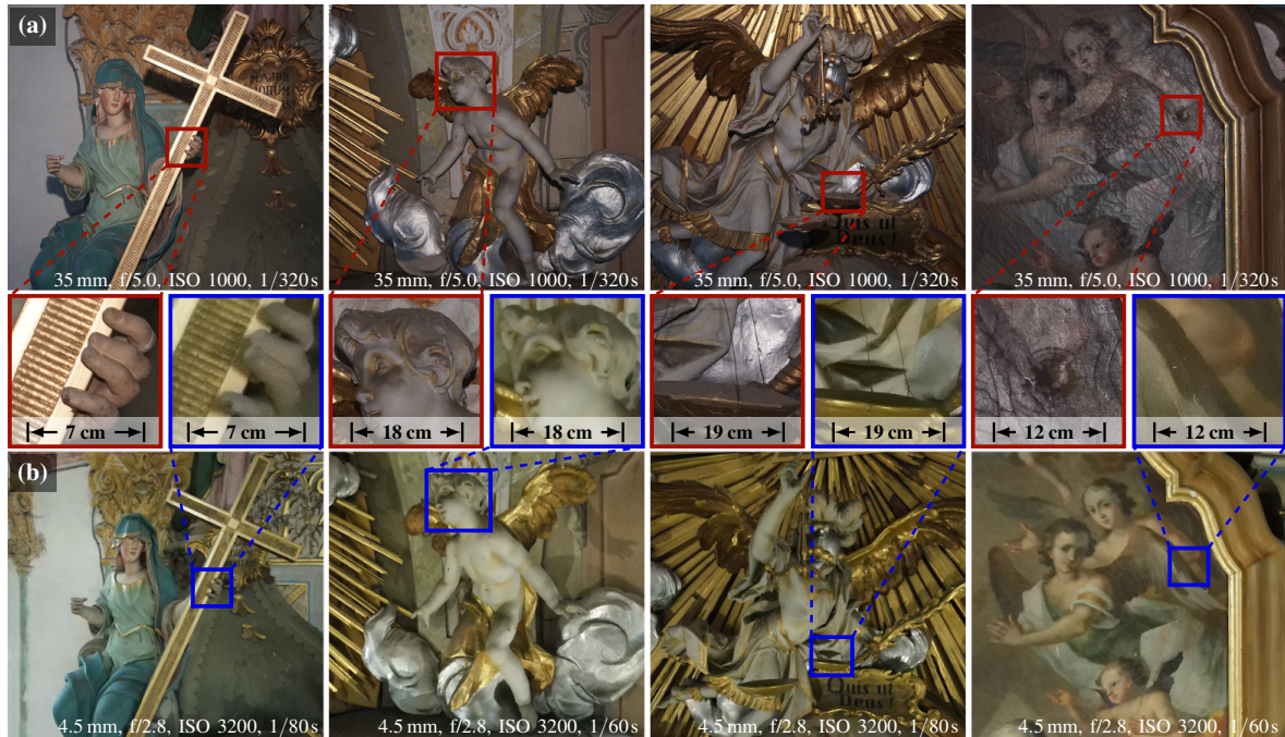
Fig. 6: Image outputs of VIS methodology as taken by the onboard MIL camera Sony Alpha A6500 (a) and commercial solution DJI Mavic Air 2 (b). Direct comparison of details of the images in the middle row shows that the proposed solution is superior in capturing high-quality details. This highlights the last column in which a hole in the painting is visible in top and absent in bottom image. Although the commercial solution is small and lightweight, its small sensor size of 6.4 \times 4.8 mm hinders usability in interior documentation.
