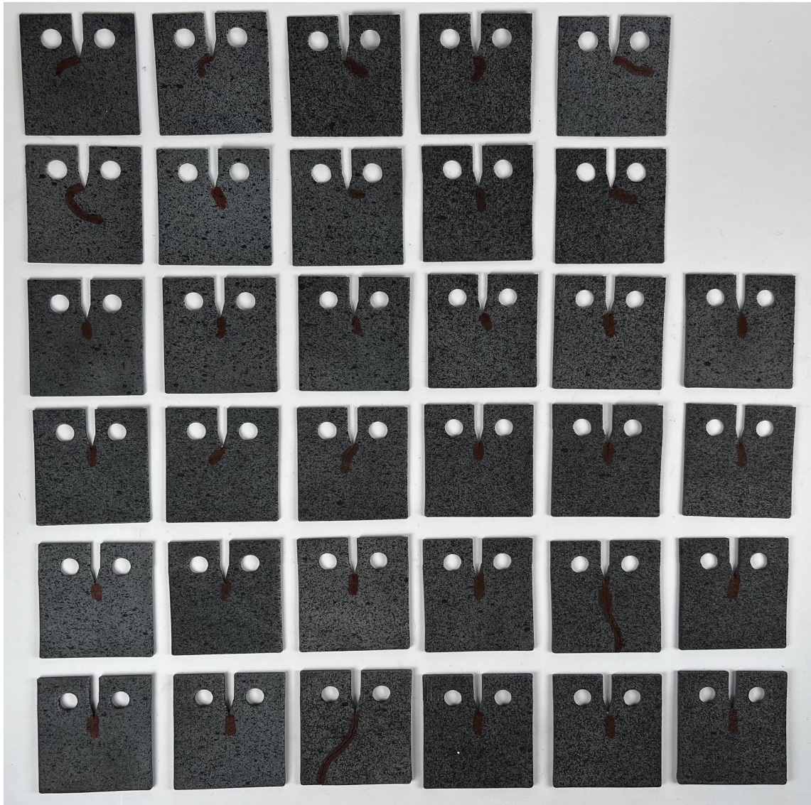
Figure 3.17: Cracks of all SAMPLE 2 for PA12 material printed in horizontal direction.
