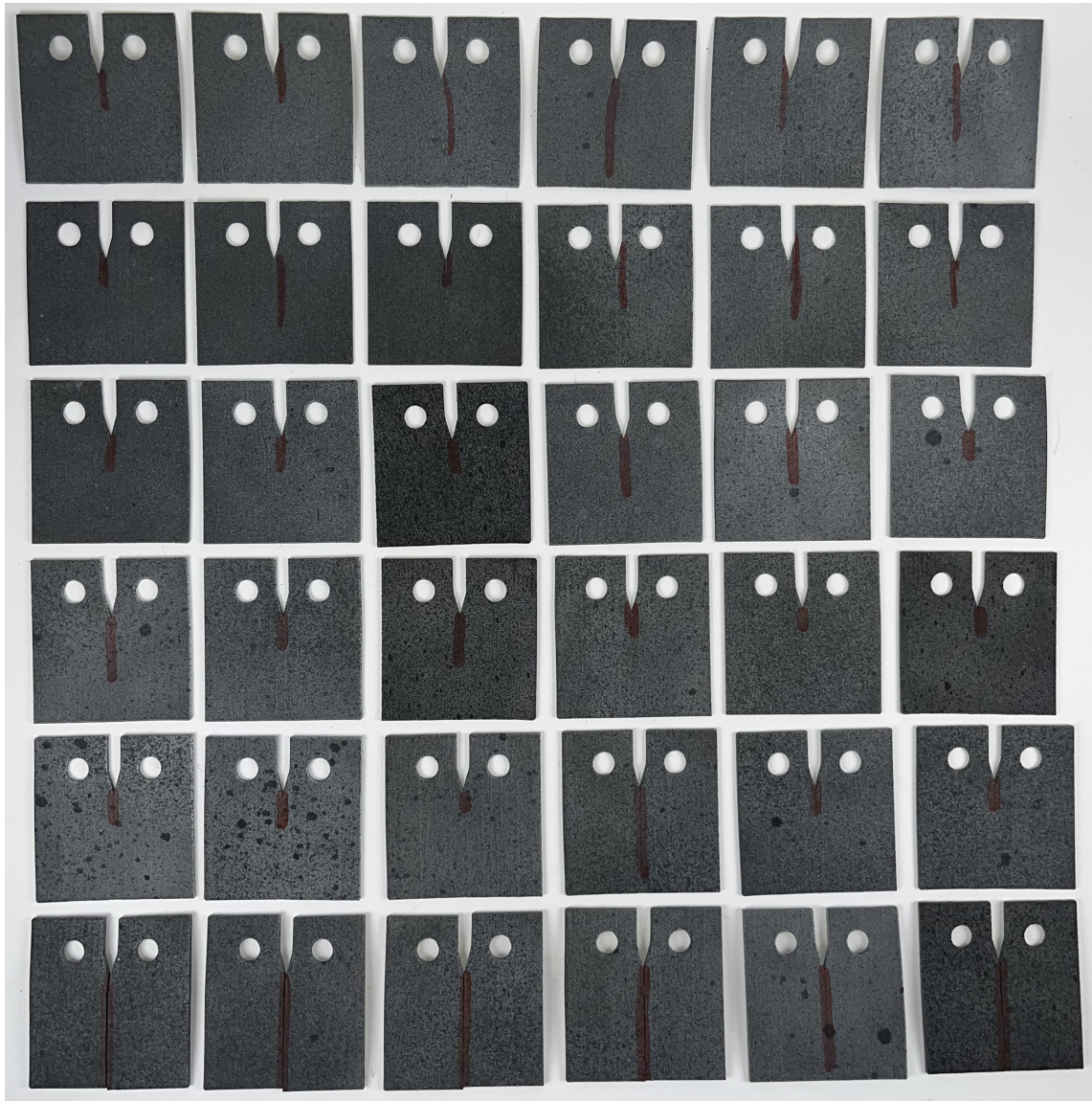
Figure 3.23: Cracks of all SAMPLE 3 for PA12 material printed in vertical direction.
