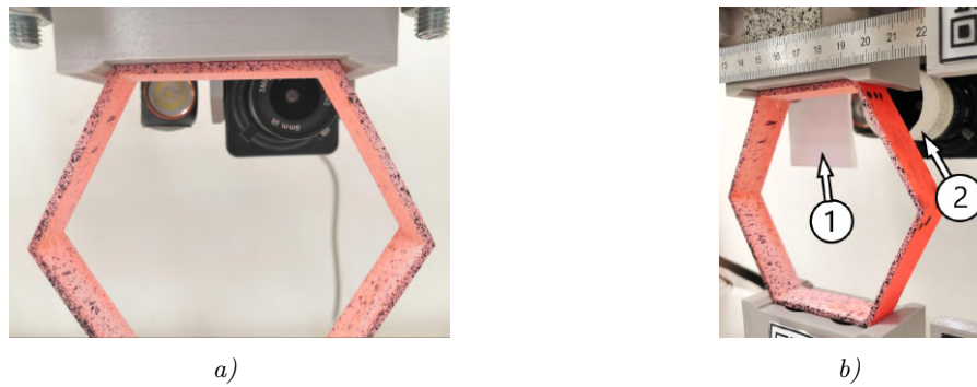
Figure 82: Experimental setup of monitoring detail region of sample, 1 - shading screen, 2 - light-dispersing shade
