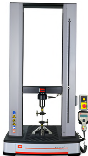
Figure 52: MTS loading machine [95]
