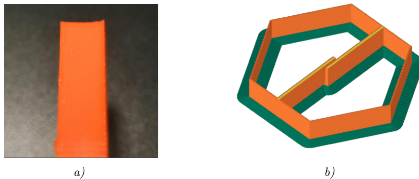
Figure 14: Deformation of vertical wall of the 3D printed sample by 0.25 mm nozzle a), Individual small hexagon cells with added supporting brim highlighted by green color b)
