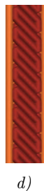
Figure 47: Infill type 2: infill at an angle of 45^\circ to the local wall coordinates. (All walls)
