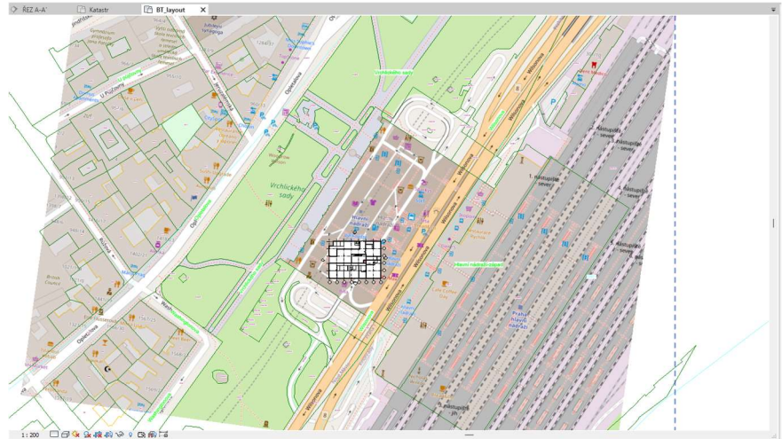
Figure 13 - Generated cadastral map in the project, the map is imported in new layout.
