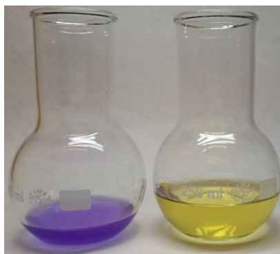
Fig. 17: Solution before and after colour change to orange - titration with HCl
