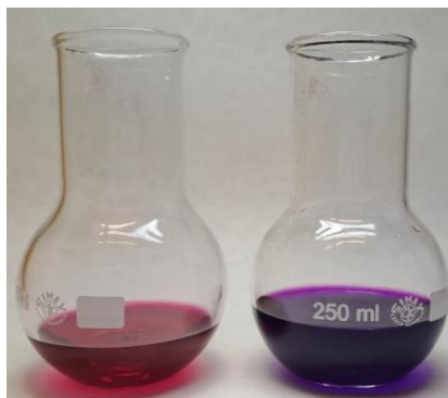
Fig. 16: Solution before and after colour change to purple - titration with EDTA
