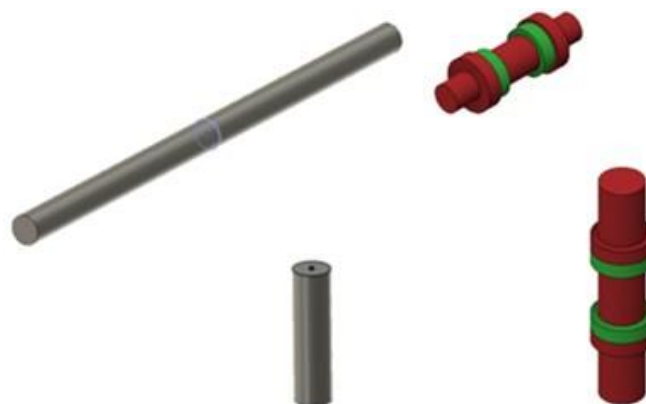
Fig. 14.: Modeling the design criteria of the bicycle part: a) region where the model will be created, b) desired and unwanted parts in the design (45)
