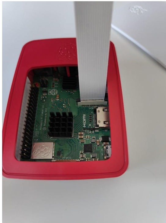
Figure 21 - Assembled Raspberry Pi with attached camera
