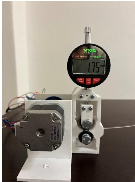
Figure 43: Thickness measuring process
