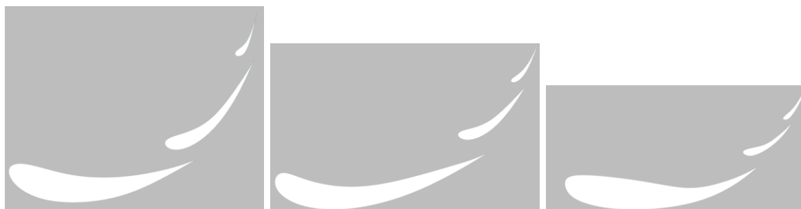
Figure 25: Aerofoil geometry for various envelopes: 520 mm – 570 mm – 620 mm
