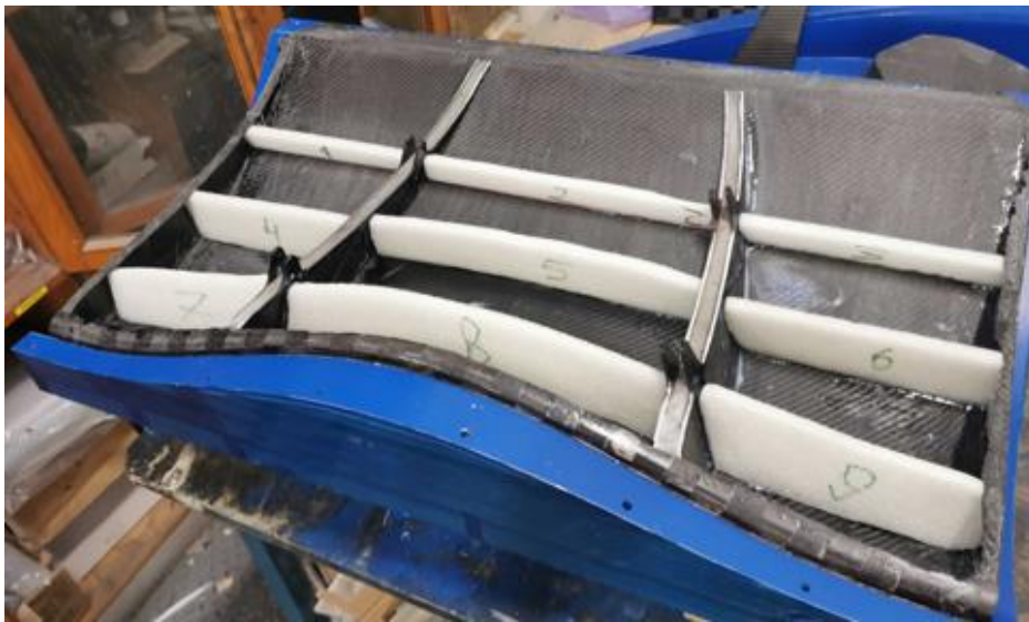
Figure 36: Inner structure of the first element of the rear wing
