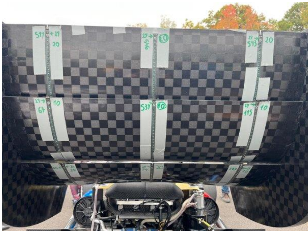
Figure 38: Pressure strips on the FS.14 rear wing
