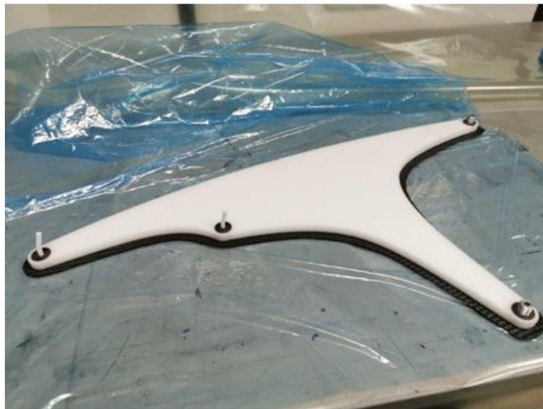
Figure 34: Rear wing holder lamination
