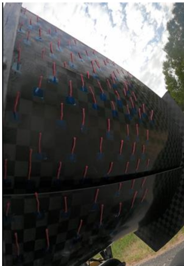
Figure 39: Cotton strings on the suction side of the FS.14 rear wing
