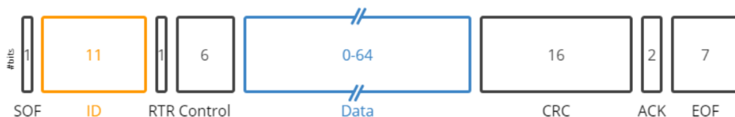
■ Figure 1.2 Structure of CAN2.0 A frame
