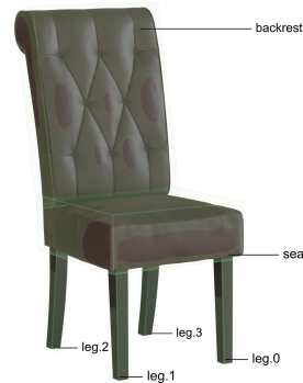
■ Figure 4.4 Example of a compound collider made out of box colliders, with simpleChair being the visible mesh and the colliders being appended to objects that are parented to the said chair
