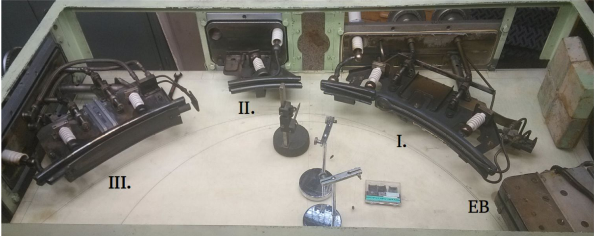
Figure 5.1: Configuration of the actual extraction system. EB – electromagnetic exciter, I. – III. Electrostatic deflectors. The beam orbits from right to left.
