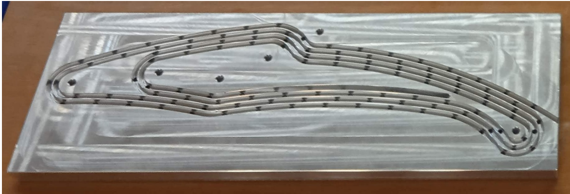
Figure 5.25: Aluminum mold for forming coils.
