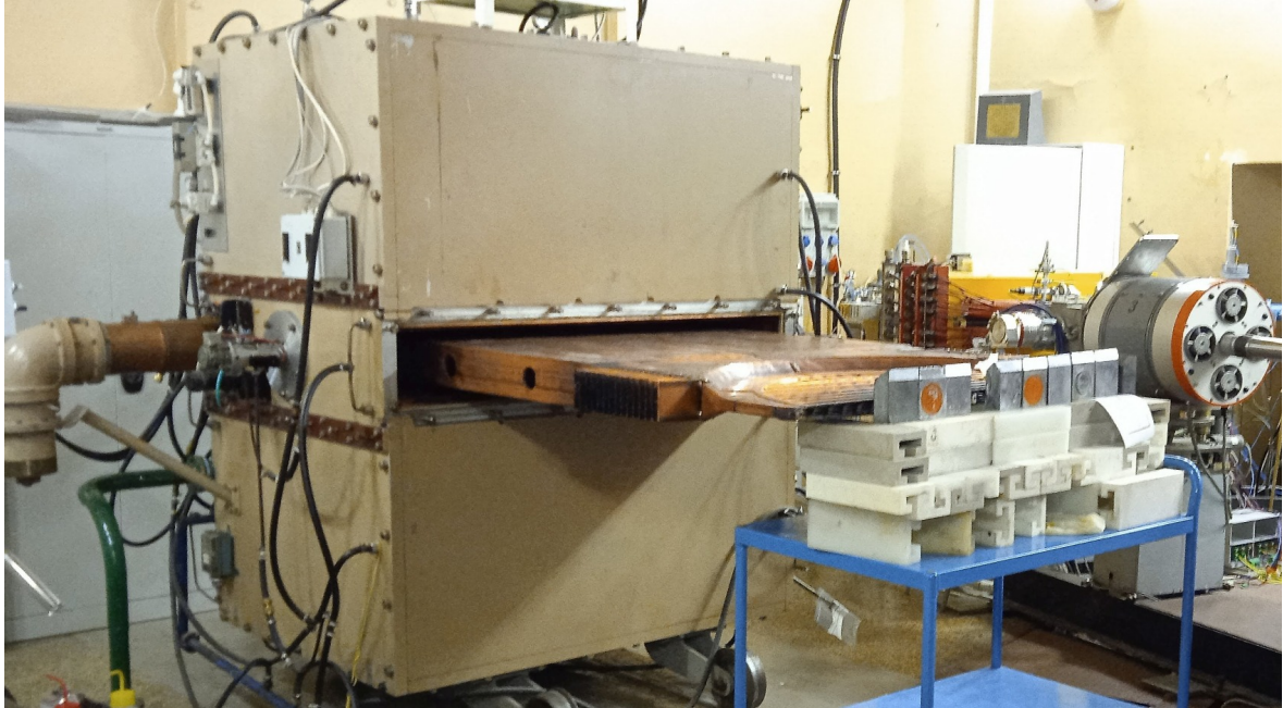
Figure 3.2: RF resonator with the dee taken out from the accelerating chamber.
