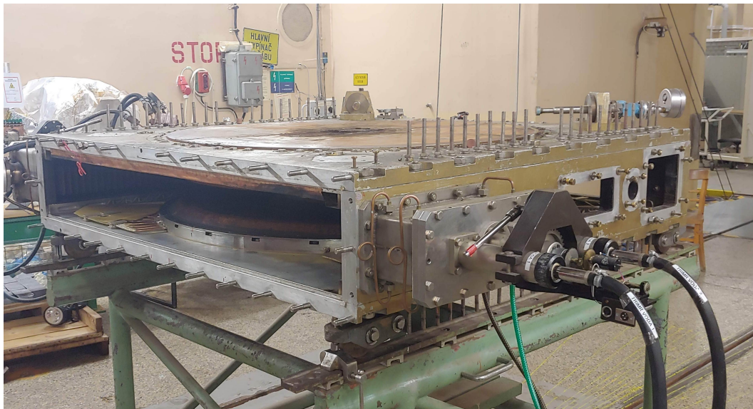
Figure 3.18: Open side of the vacuum chamber.
