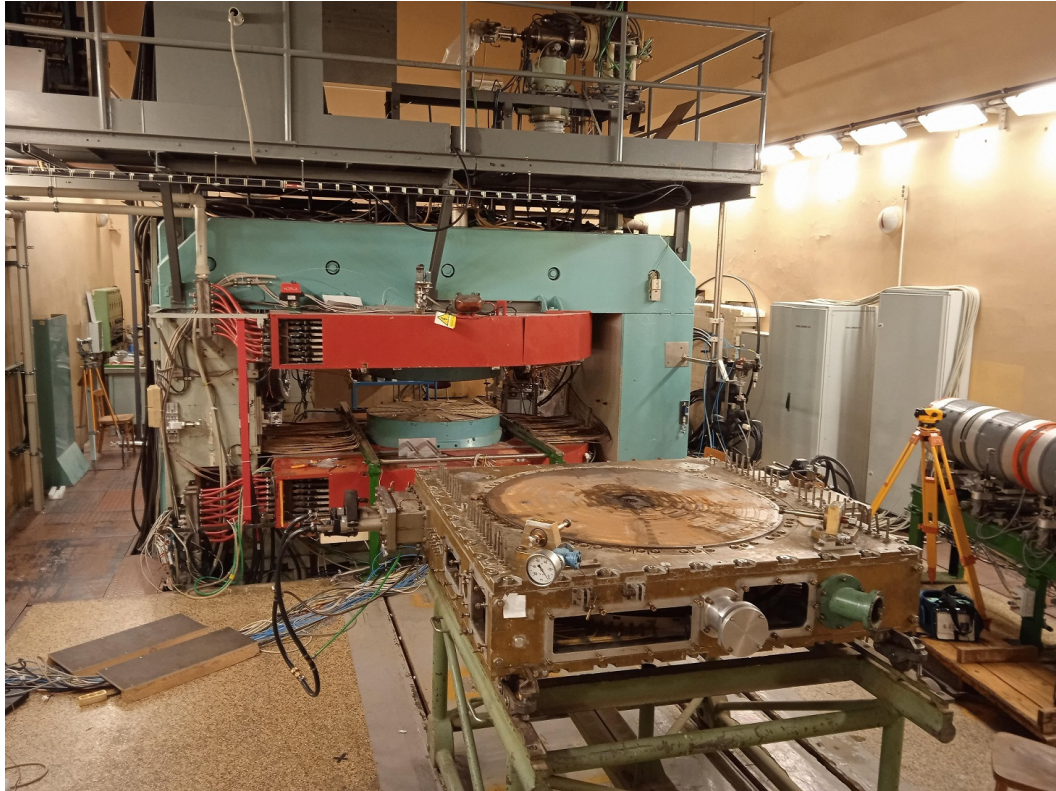
Figure 3.17: Vacuum chamber pulled out from the cyclotron magnet.
