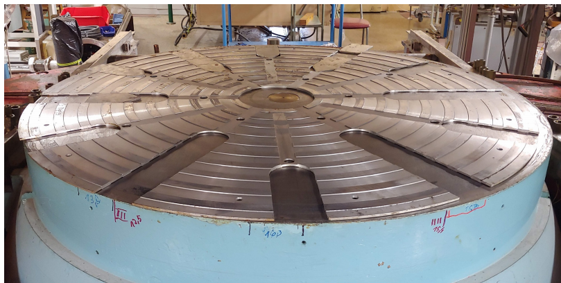
Figure 3.28: Alumina flake disk with cutouts for the ferromagnetic inserts.
