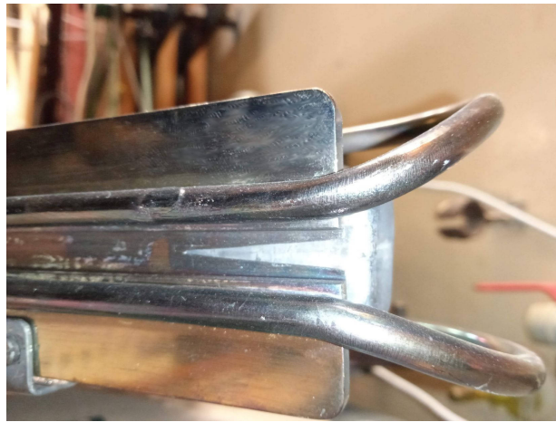
Figure 5.5: V-shaped beginning of the first deflector electrostatic septum.
