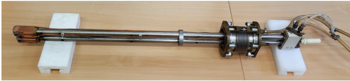
Figure 3.3: Internal U-120M PIG ion source.
